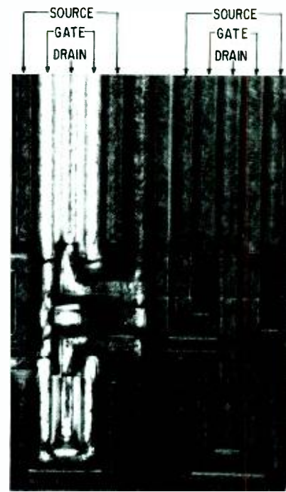
Fig. 1 — Operation of COS/MOS circuit with left transistor pair functioning and right transistor pair quiescent. Location of source, gate, and drain electrodes that constitute a MOS transistor are indicated.
