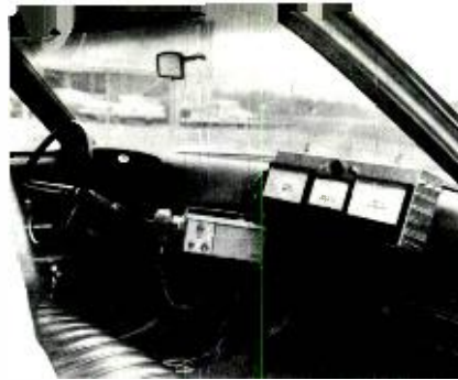
Fig. 16 — Processing and display unit inside vehicle.
