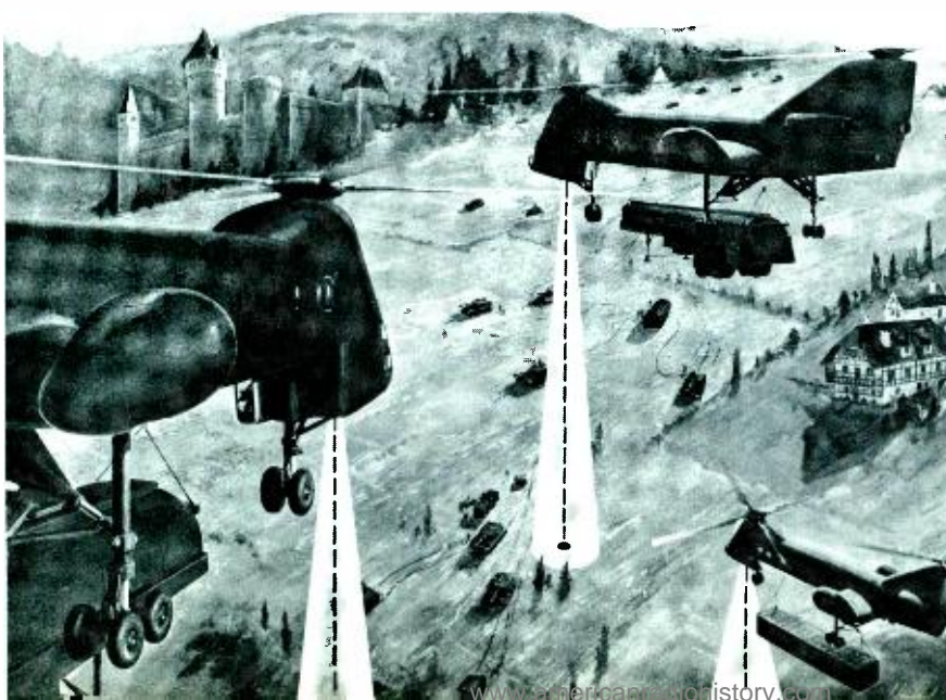
Fig. 1—Precision hover sensor beam patterns from the helicopter.
