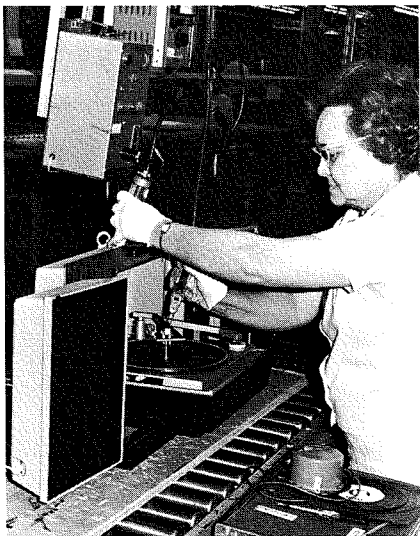
Fig. 5—UL-required "Hi-Pot" test equipment in use on an assembly line (Indianapolis).
