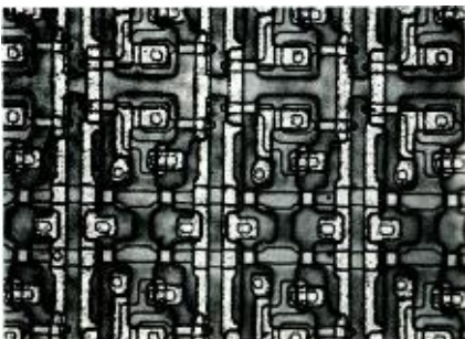
Fig. 4—Beam-lead, silicon-gate PMOS memory array.
