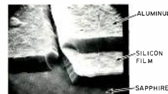
Fig. 8—Continuous aluminum at SOS step.
