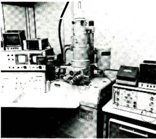
Fig. 4—Scanning electron microscope used in the diagnosis of faults in solid-state devices and integrated circuits.
