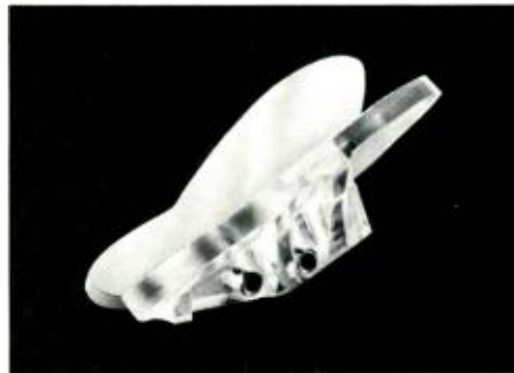
Fig. 4—Roof or Amici mirror. This butterfly-shaped, quartz, front-surfaced mirror deflects the line-of-sight by 45^\circ and re-inverts and re-reverts the image from the lens to provide an upright, properly oriented image on the viewing screen.
