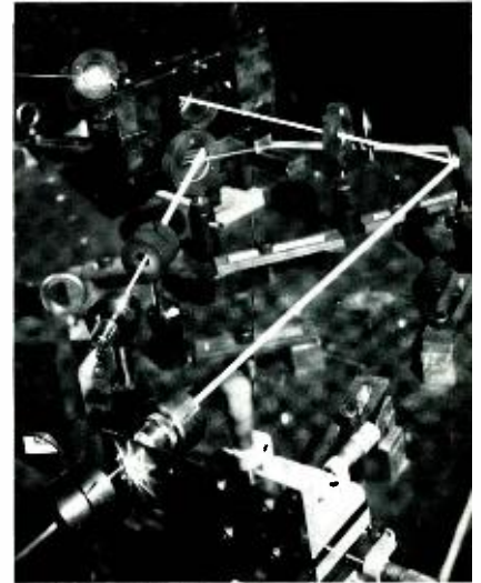
Research and development programs in laser technology and holography led to many new concepts and products. The photo shows one method used for constructing a hologram. An argon laser beam (top, left) enters an optical obstacle path where it is split into two beams by a half-silvered mirror and sent along separate paths to become the object and reference beams required to produce a hologram. The beam on the left is the object beam and can be seen to diverge into a cone just before it strikes the object (a transparency) to be holographed.
