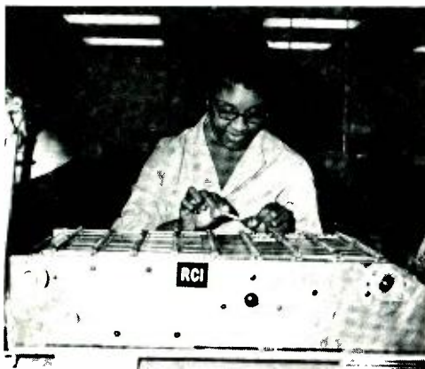
A hot-plate system for reflow joining.
