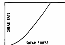
c) Non-newtonian pseudo-plastic: beyond a given rate of shear, permanent physical deformation will result and resistance to flow will be independent of rate of shear.
