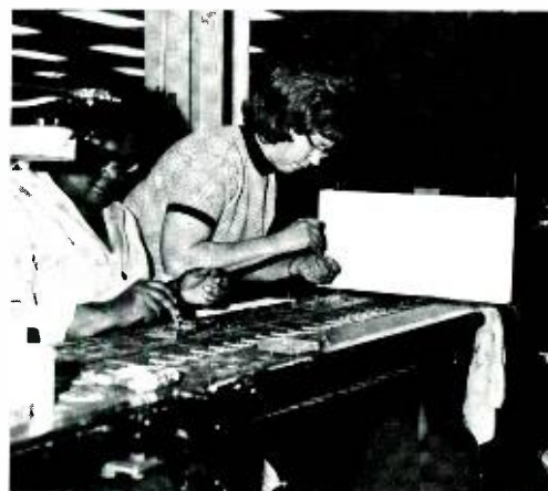
Components being placed on circuit boards. Flowing of the paste and component joining are accomplished in one operation in the infrared oven.
