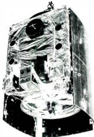
Fig. 7—ITOS-1 spacecraft with solar panels folded back in the launch configuration.
