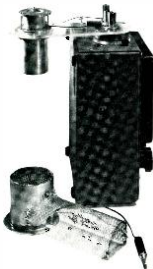
Fig. 1—Device for making triboelectric measurements.
