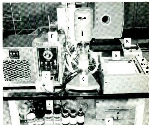
Fig. 2—The Ferranti-Shirley cone and plate viscometer: A) X-Y recorder, B) control and indicator unit, C) measuring unit, D) automatic gap-setting unit, E) amplifier unit, F) constant temperature water bath.
