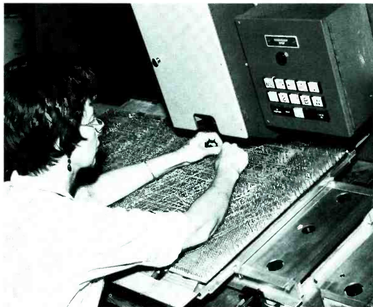
Semi-automatic wire-wrap machine.
