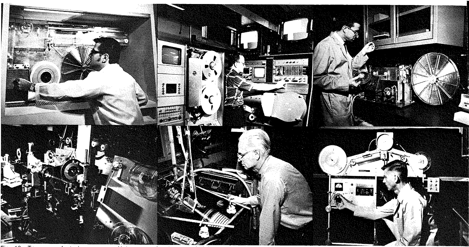
Fig. 12—Tape manufacturing process. Holograms of color encoded images are recorded on photoresist coated tape; Ni master tape is fabricated from the original holographic tape and used to emboss vinyl replicas. Clockwise from top left: Fig. 12a—coating; Fig. 12b—encoding; Fig. 12c—recording; Fig. 12d—developing; Fig. 12e—plating; and Fig. 12f—replicating.
