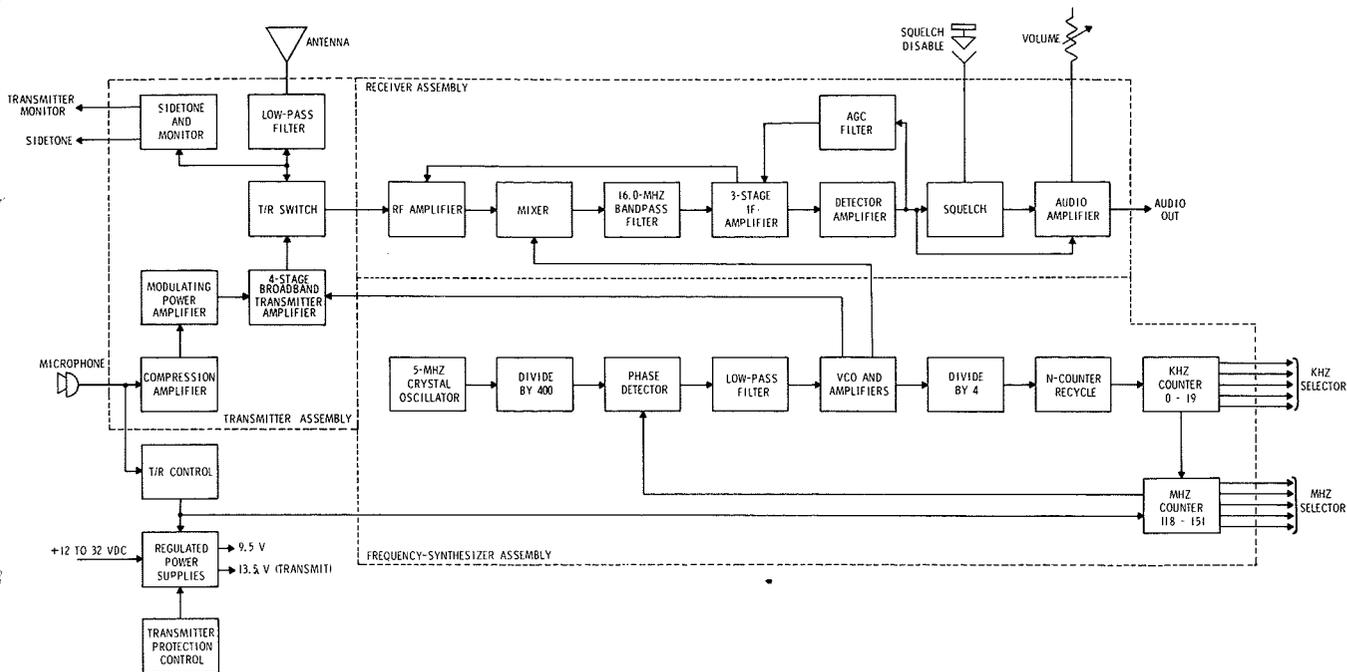
Fig. 1—AVC-110 VHF Communication Transceiver; the heart of this unit is the digital frequency synthesizer which provides precise RF signals for both transmitter and receiver.
