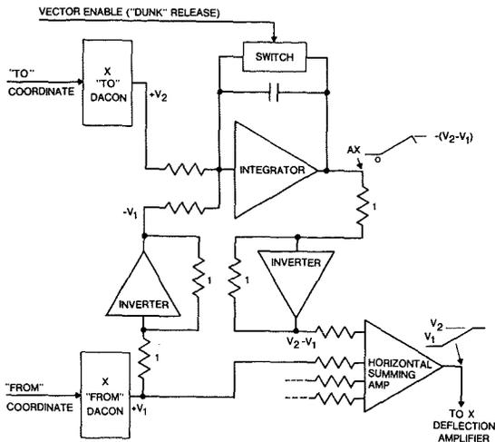
Fig. 3—Simplified block diagram of the horizontal vector generator.
