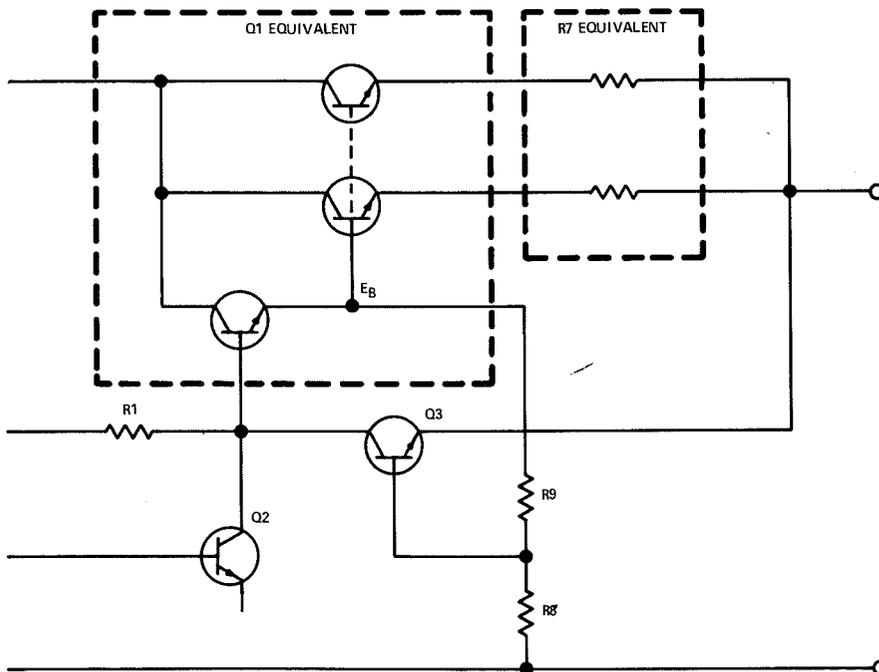
Fig. 7—Alternate configuration for foldback current limiting.
