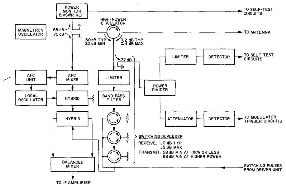
Fig. 4—Block diagram of microwave system.
