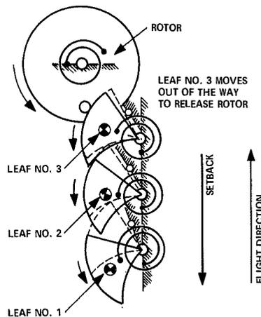
Fig. 2—First-order integrating accelerometer.
