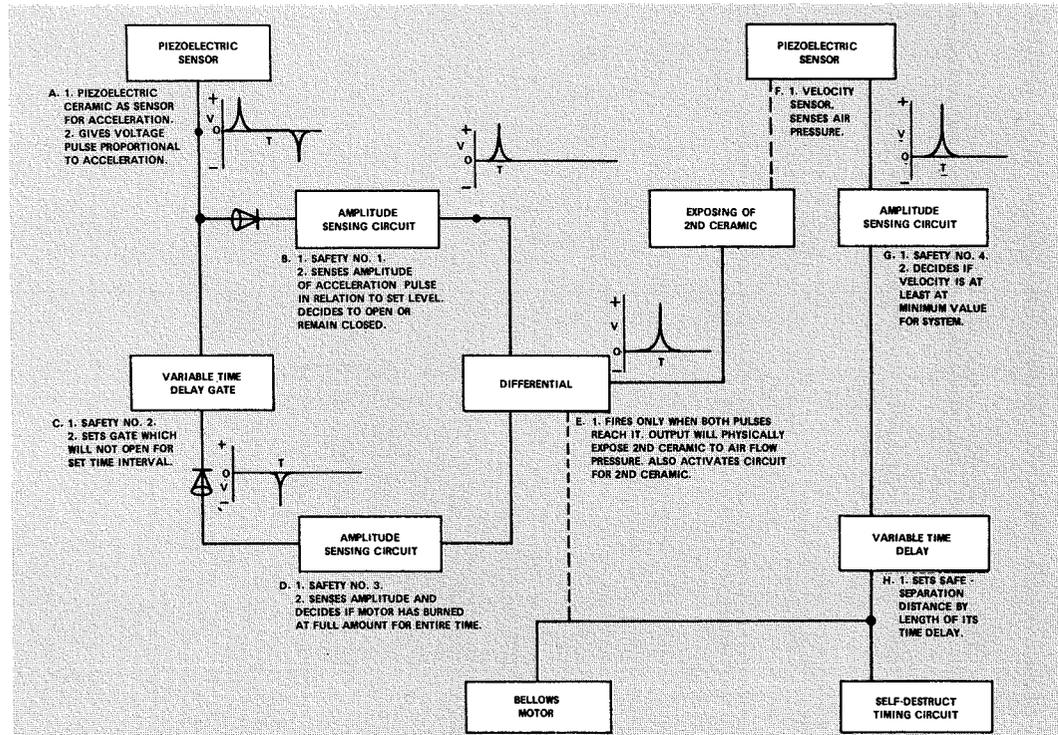
Fig. 6—Electronic safety-and-arming device.
