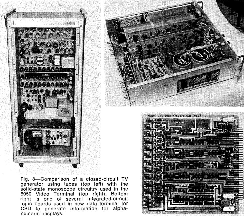
Fig. 3—Comparison of a closed-circuit TV generator using tubes (top left) with the solid-state monochrome circuitry used in the 6050 Video Terminal (top right). Bottom right is one of several integrated-circuit logic boards used in new data terminal for CSD to generate information for alpha-numeric displays.
