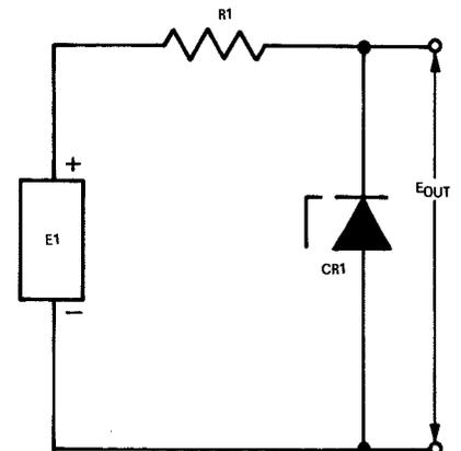
Fig. 1—Basic voltage-regulated supply.
