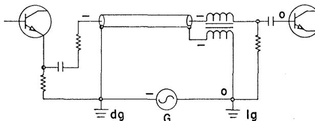
Fig. 2—Video hum voltage bucked out by transformer.
