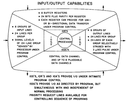
Fig. 5—RCA-110A input/output capabilities.
