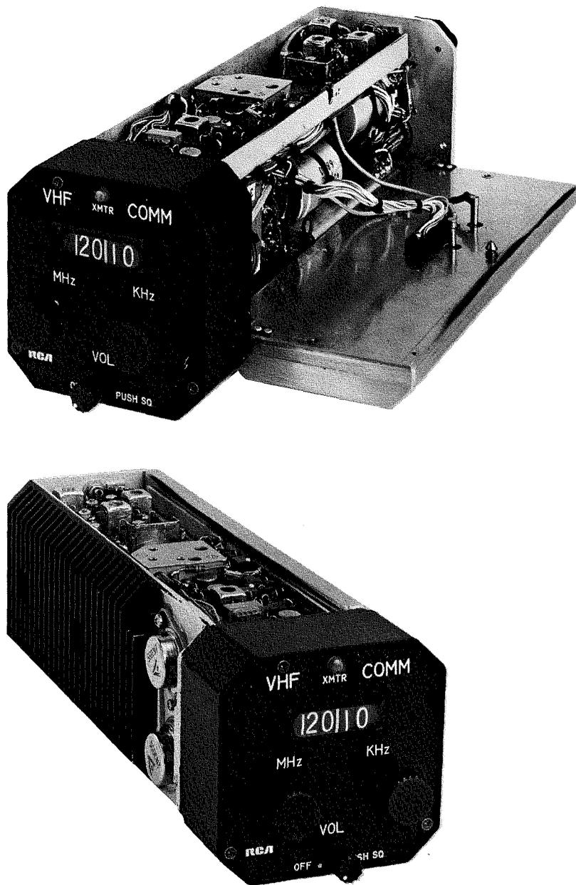
Fig. 2—The AVC-110 transceiver package weighs only 4.8 lbs., is 3x3x10 inches in size, yet delivers 20W of transmitter power for a rated 200-n mi. range.
