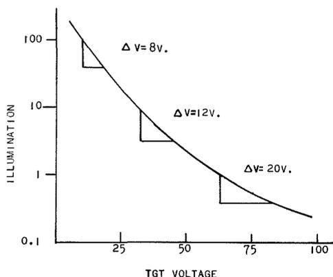
Fig. 7—Constant signal-current characteristic for a typical vidicon.
