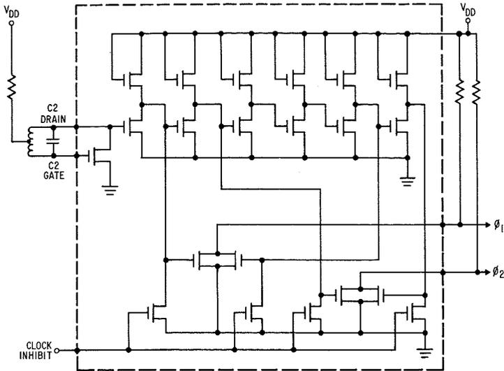
Fig. 4—Two-phase clock circuit.
