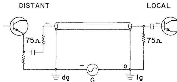
Fig. 1—Hum voltage in video by AC ground potential difference showing phase relationship from G.
