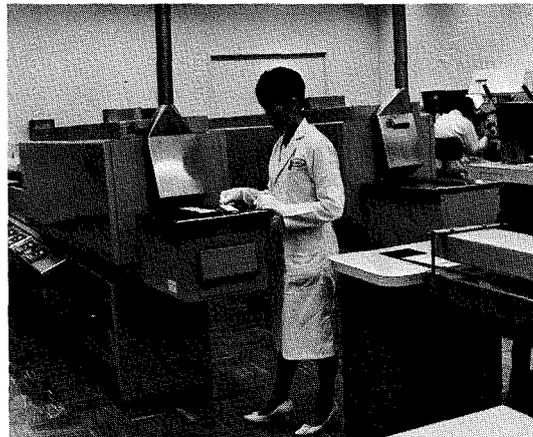
Fig. 4—Furnace equipment for firing substrates.
