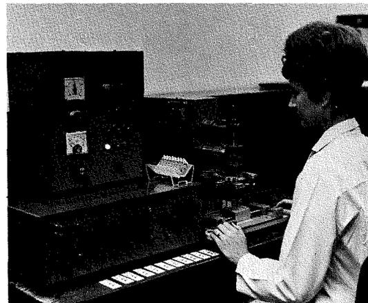
Fig. 5—Resistor trimming by sand abrasion.
