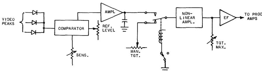
Fig. 6—The automatic-target circuit uses a non-linear amplifier to create a linear closed-loop servo system.
