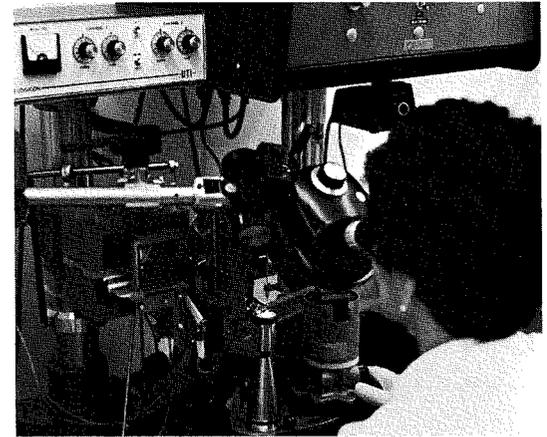
Fig. 8—Die-attach equipment for chip mounting.
