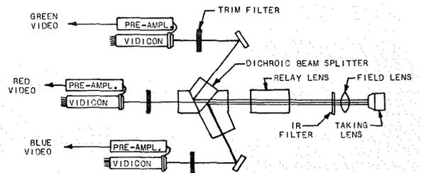
Fig. 2—Relay optical system and dichroic beam-splitter assembly.
