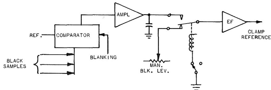
Fig. 5—Automatic black-level circuitry which serves the clamping reference for the processor amplifiers.
