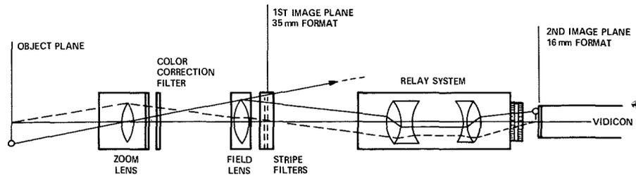
Fig. 6—Optics of 1-vidicon color camera system.
