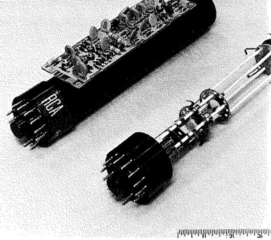
Fig. 1—In the external view on the left, the circuit board on top of the monoscope tube is the video pre-amplifier; to the right is the internal structure including socket, deflection plates, character stencil (target), and signal electrode.
