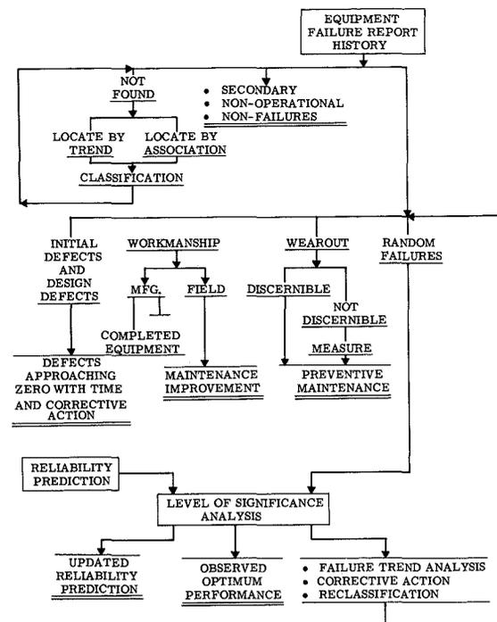
Fig. 3—Failure report classification and use.
