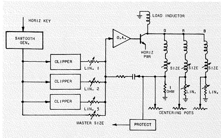
Fig. 9—The horizontal deflection amplifier uses a non-linear reference sawtooth to create a linear scan.
