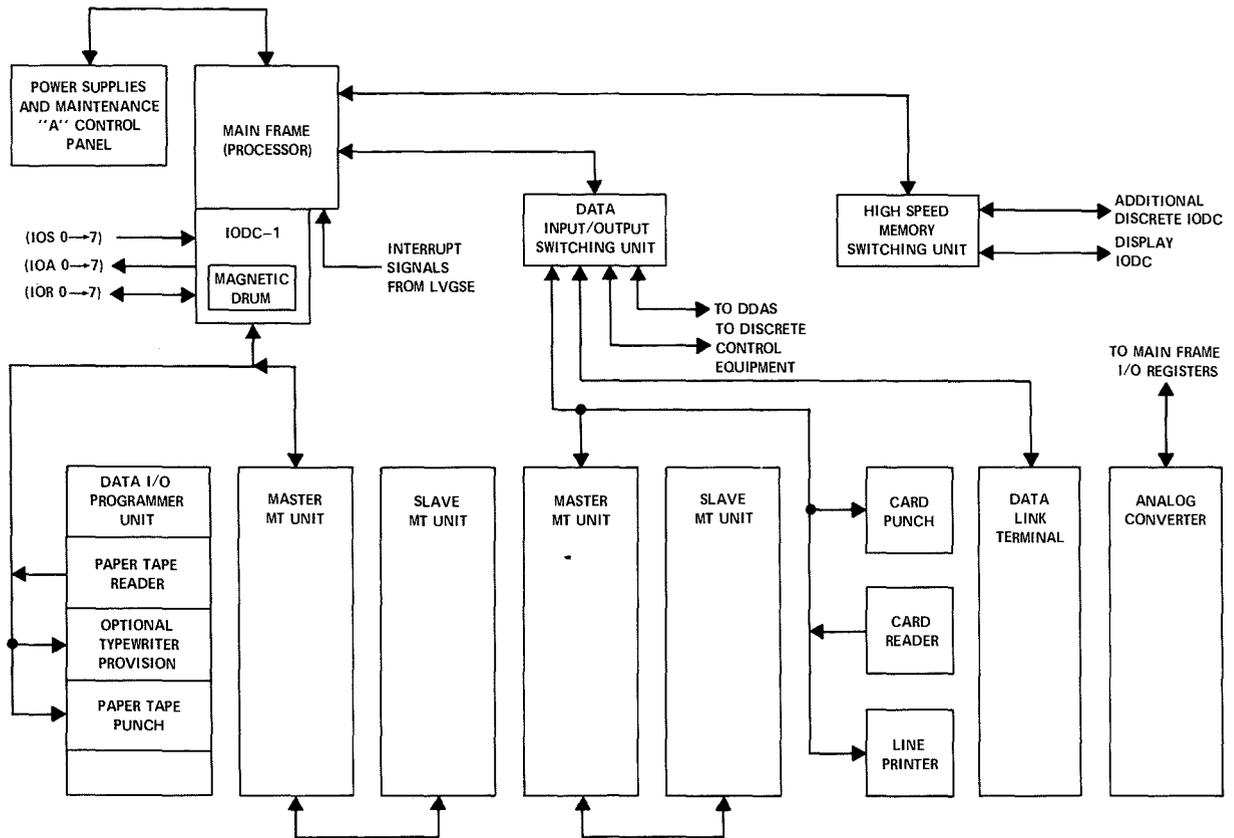
Fig. 2—The RCA-110A computer equipment interconnection.
