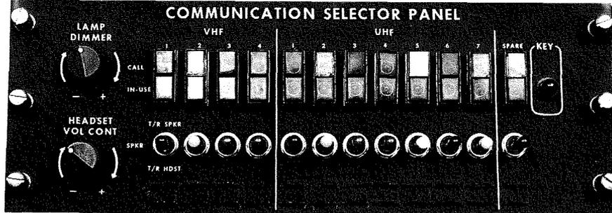
Fig. 5—Communications selector panel.
