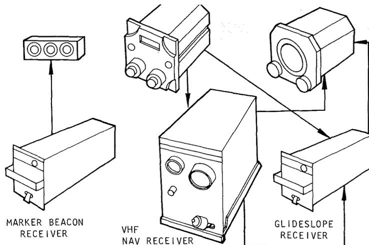
Fig. 2—Typical navigation system with traditional remotely-mounted black boxes before the introduction of the AVN-210.
