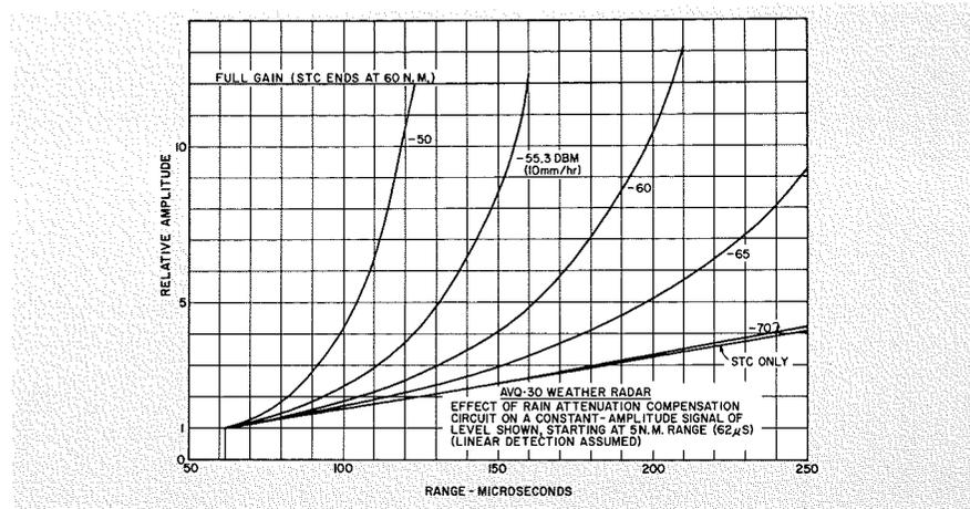
Fig. 5—Gain versus range in rain-attenuation-compensation circuit operation.
