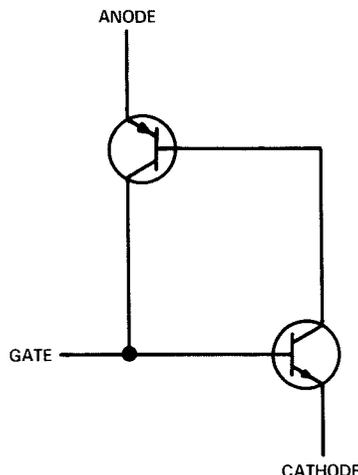
Fig. 4—This transistor pair can replace the SCR shown in Fig. 3.
