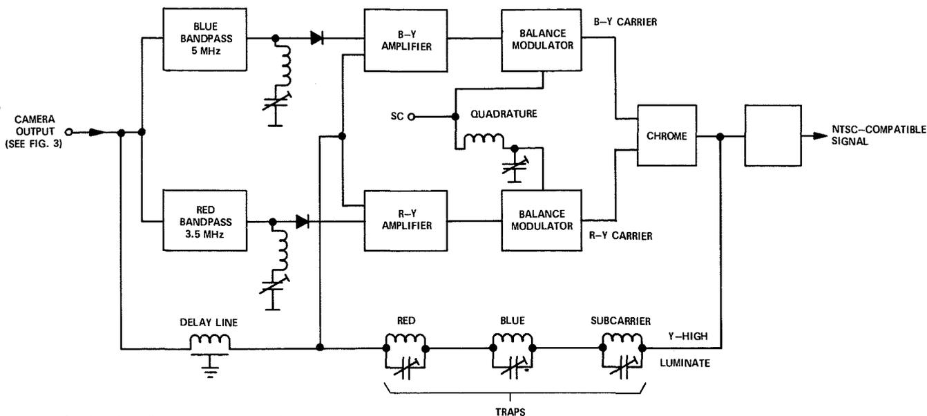
Fig. 5—Carrier detection and color encoding.
