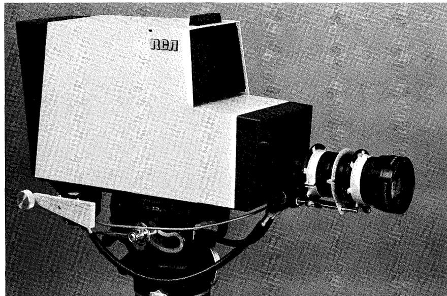
Fig. 1 (above)—One-tube color camera.
