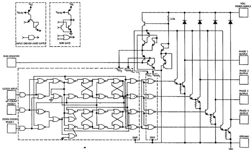
Fig. 1a—Logic and simplified circuit diagram for motor controller.
