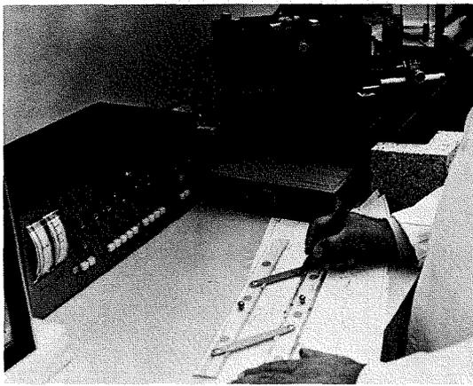
Fig. 2—Thick-film deposition analyzer.
