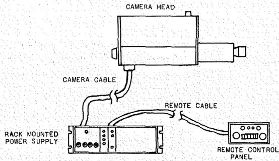
Fig. 1—System components for economical color film camera.
