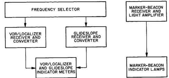
Fig. 2—Grouping by black box of airborne VOR/ILS receiver functions before RCA's AVN-210 system.
