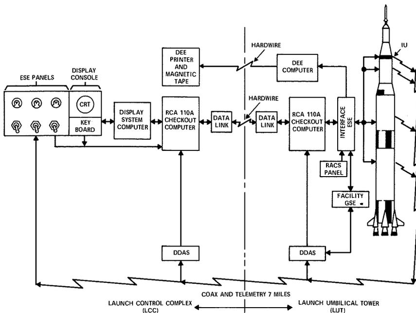
Fig. 4—Equipment interconnection for prelaunch checkout and launch control.
