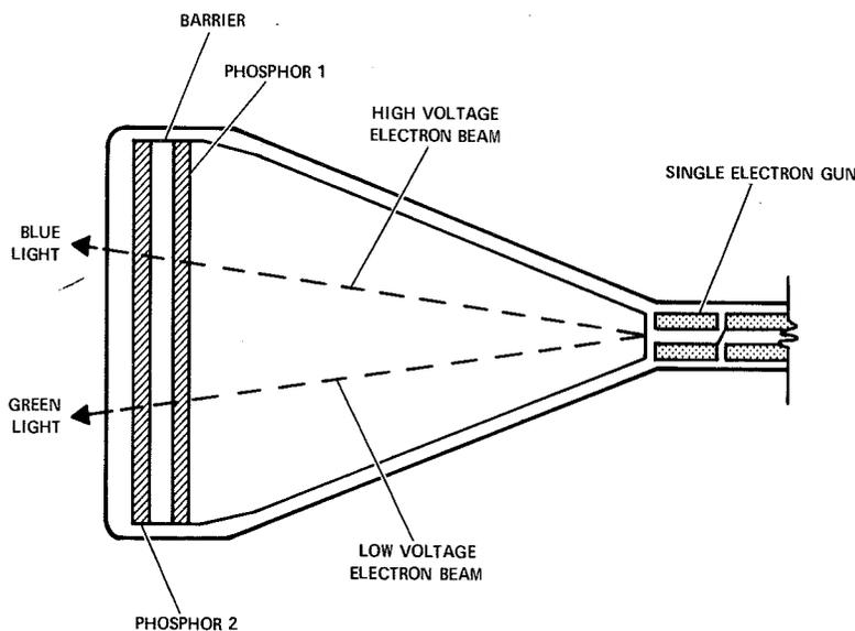
Fig. 1—Conventional two-color layered-phosphor CRT.
