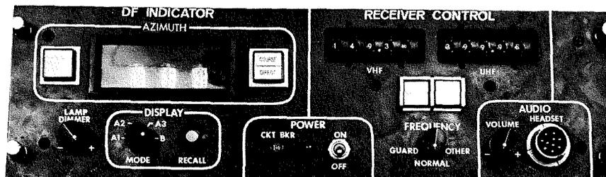
Fig. 3—RDF Display/Receiver Control Panel.
