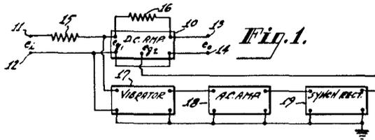
Fig. 2—Block diagram of E. A. Goldberg's patent for stabilized DC amplifier—a big assist for analog computers.
