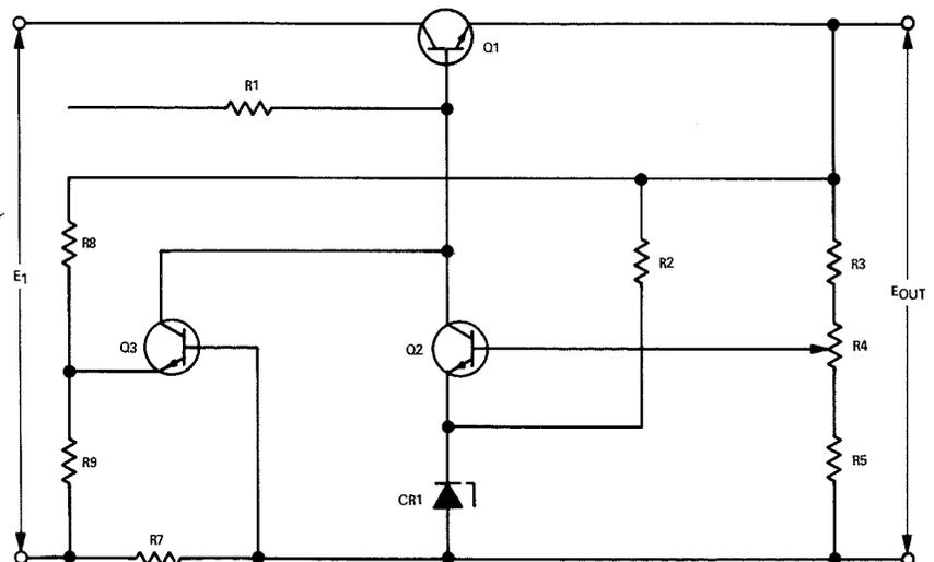
Fig. 5—A supply with foldback current limiting.
