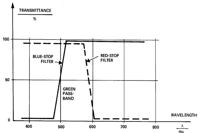
Fig. 4—Idealized dichroic-filter curves.
