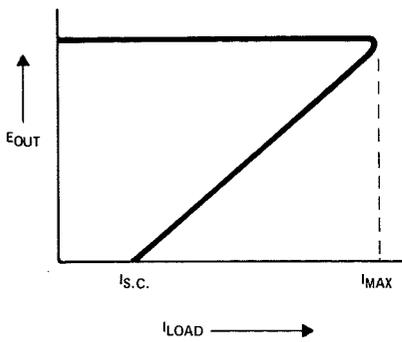
Fig. 6—Characteristics of foldback current limiting.
