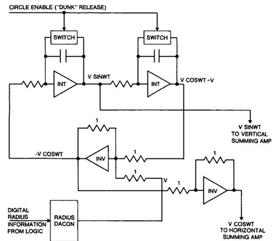
Fig. 4—Simplified block diagram of the circle generator.
