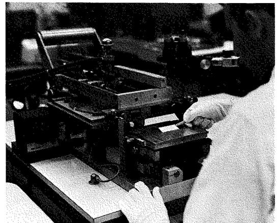
Fig. 1—Precision printer for fabricating thick-film networks.
