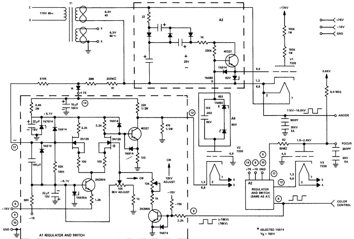
Fig. 3—High-voltage switching for the two-color display.
