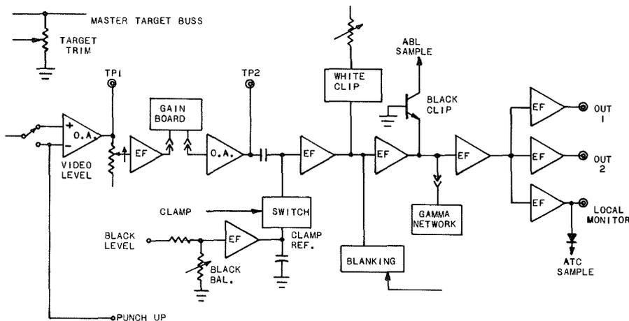
Fig. 4—Processing amplifier showing setup adjustments and plug-in submodules.
