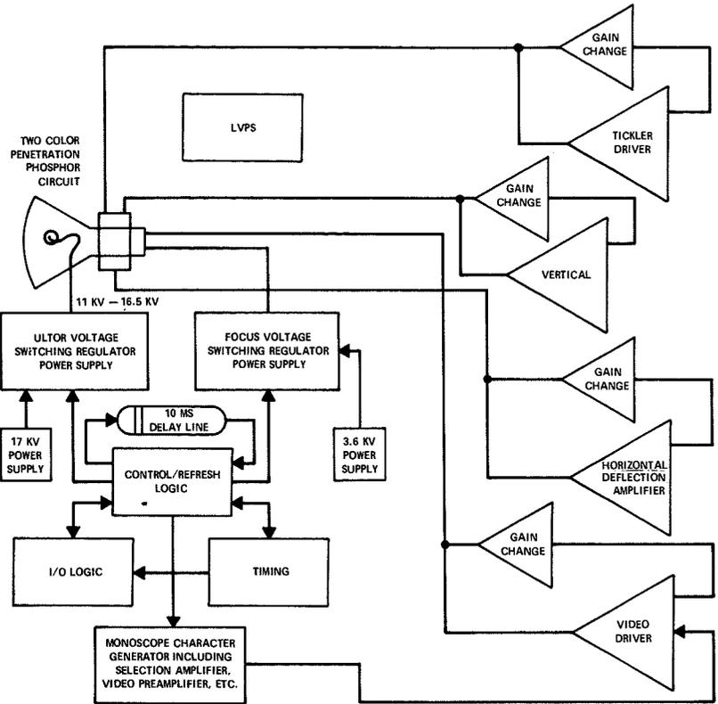
Fig. 2—Simplified block diagram of the two-color display.
