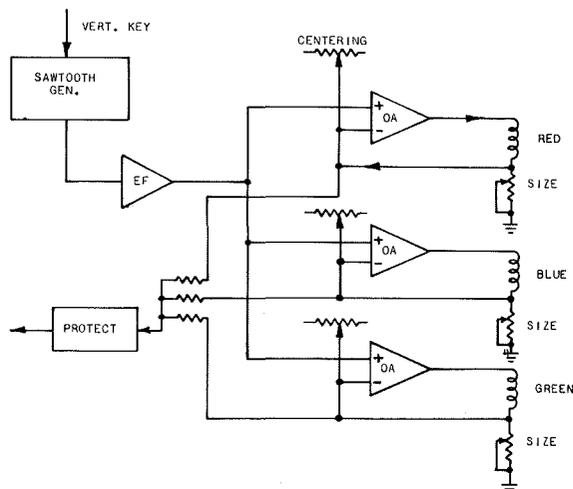
Fig. 8—The three vertical deflection yokes are each individually driven by a current feedback sweep amplifier.
