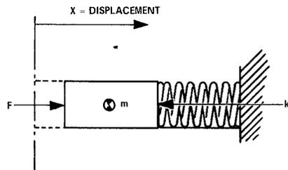
Fig. 1—Basic mass and spring system.
