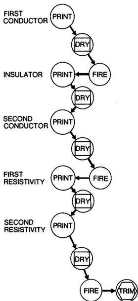
Fig. 6—Simplified process flow diagram for multilayer fabrication.
