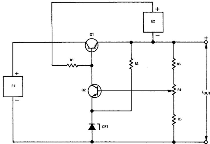
Fig. 2—Basic voltage-regulated supply.
