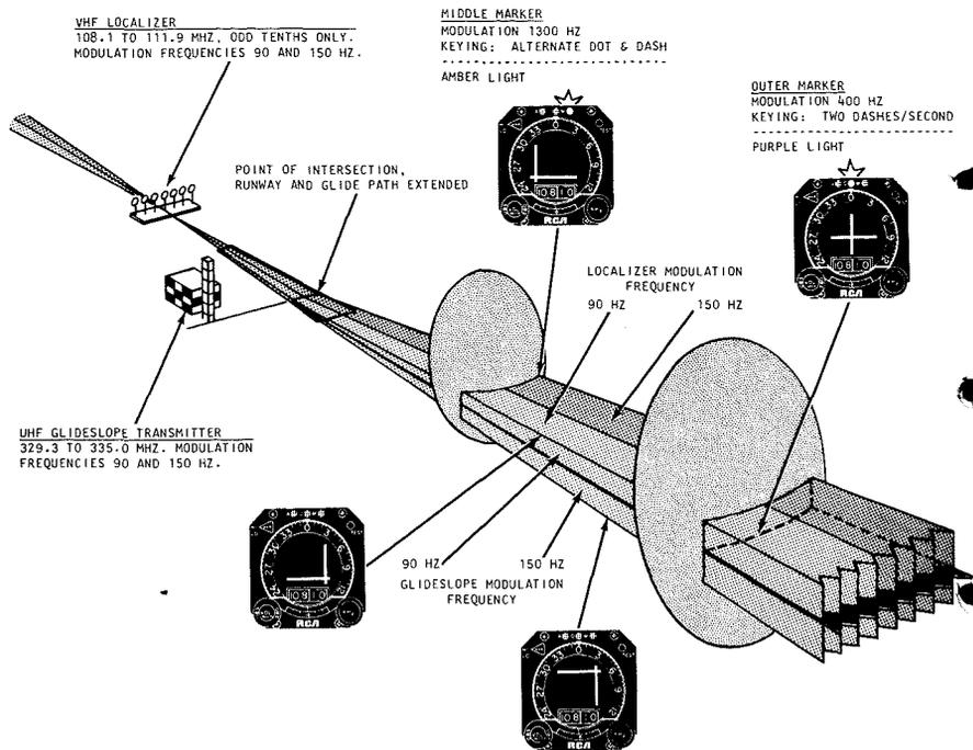
Fig. 1—Instrument landing system.
