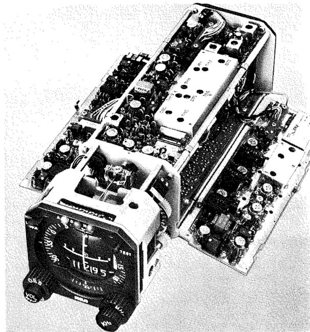
Fig. 4—All AVN-210 subsystems are accessible for servicing.
