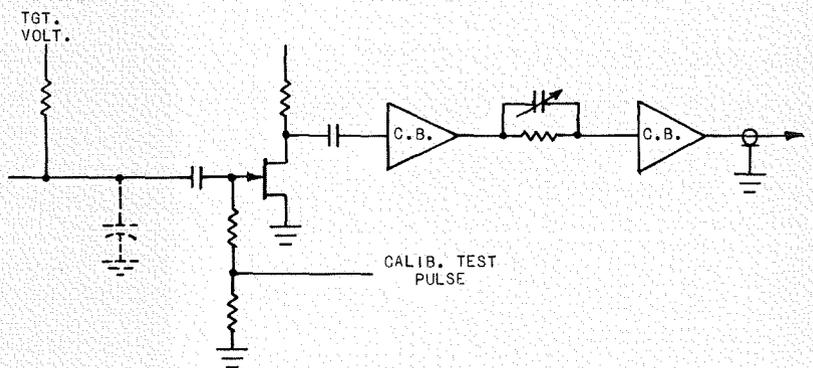
Fig. 3—Preamplifiers use a FET for low-noise performance. The calibrated test pulse serves as an aid in setting signal current levels.
