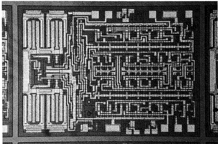
Fig. 1b—Magnified view of monolithic motor control circuit chip.
