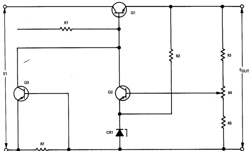
Fig. 3—Supply with foldback current limiting.
