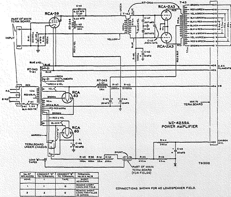
Fig. 1—Power amplifier schematic using RCA80, 83, and 2A3 tubes. The amplifier was part of the RCA Photophone Theater Sound System of the 1930's.
