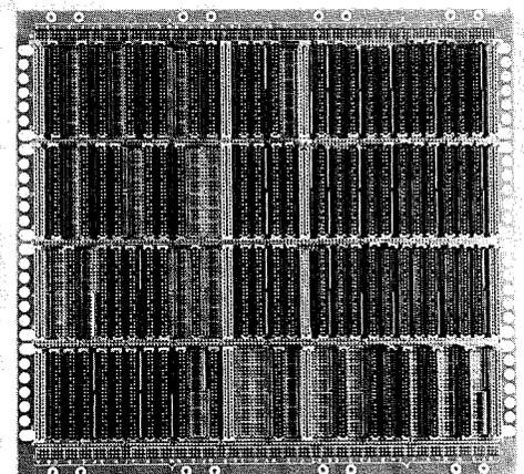
Fig. 7—Backplane that was designed by a computer for the 4101C computer.
