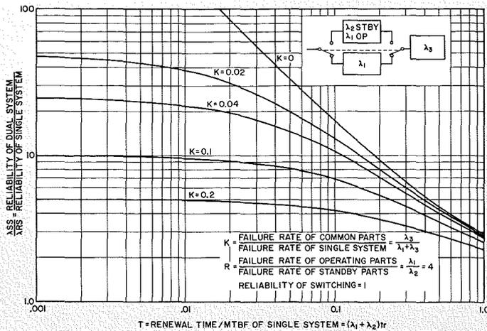
Fig. 3—Single-system versus dual-system reliability.
