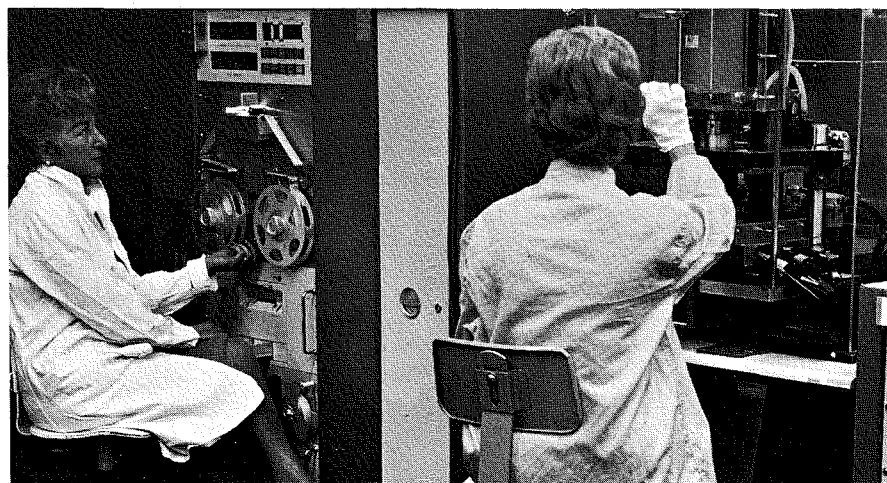
DIT-MCO 6120 for testing unpopulated printed-circuit boards.
