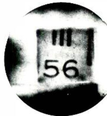
Fig. 15—Image of numerals seen through a GaAs crystal.
