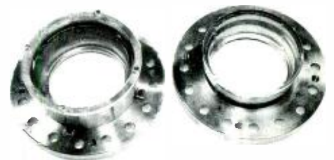
Fig. 8—Bakeable UHV five-inch windows, utilizing optical quality glass are supplied by ECD in Lancaster, Pa. Spectral transmission from 3,000 to 30,000 angstroms.
