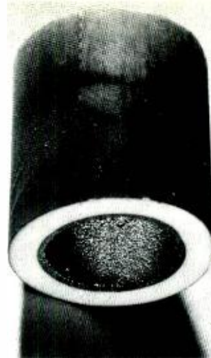
Fig. 5—Vapor-deposited Nb 3 Sn on the inside of a ceramic cylinder.
