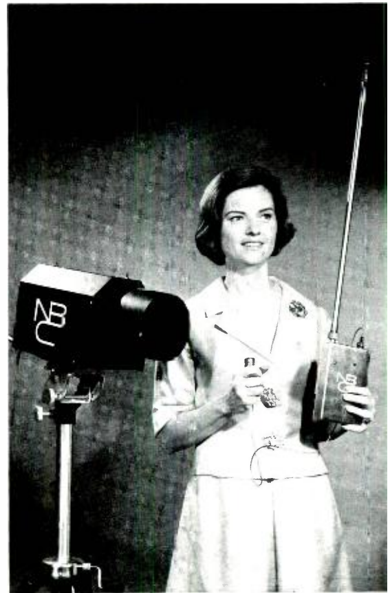
Fig. 3—At left is the black-light receiver and (right) is the hand-held black-light transmitter.
