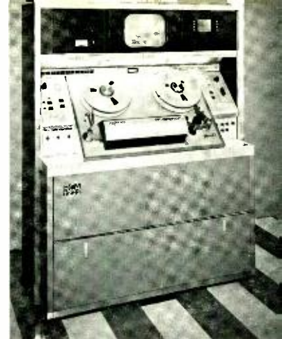
Fig. 6—The TR-22, industry's first all-transistor TV tape recorder; size is again substantially reduced and reliability improved.
