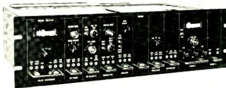
Fig. 8—TRT-1 pixlock servo control unit stabilizes the mechanical scanning within \pm 100 nsec.
