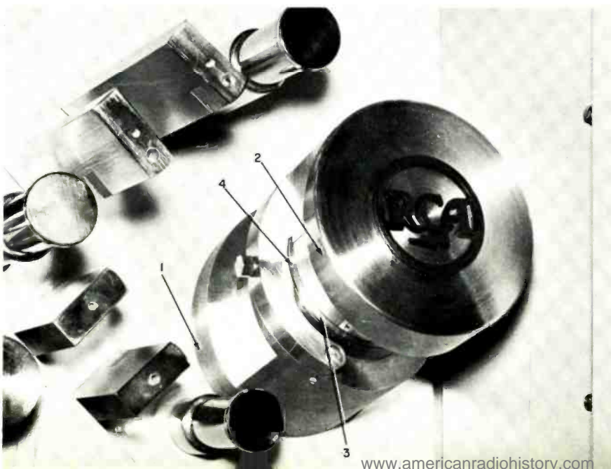
Fig. 2—Helical-scan headwheel assembly (closed).
