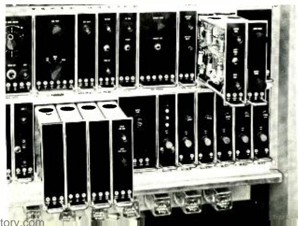
Fig. 14—The six color ATC modules for TR-22, shown partially withdrawn.
