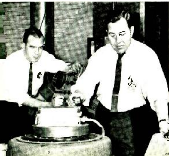
Fig. 3—G. S. Newcomb (left), and E. R. Ware conduct an environmental test in the Camden Environmental Test Facility to check performance under extensive vibration, equivalent to that of the spacecraft re-entry phase.
