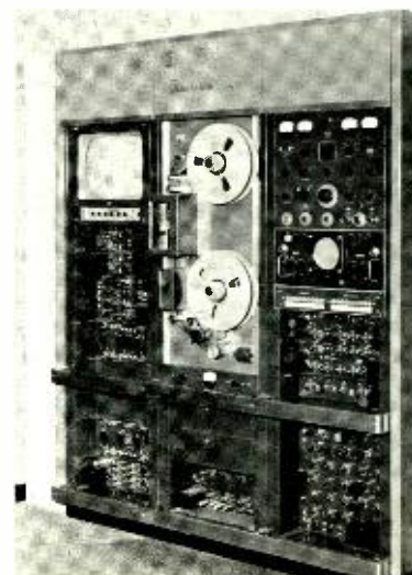
Fig. 3—TRT-1A first production-model TV tape recorder: five racks were used; left photo shows signal, transport and control racks; right photo shows power supply and servo racks.
