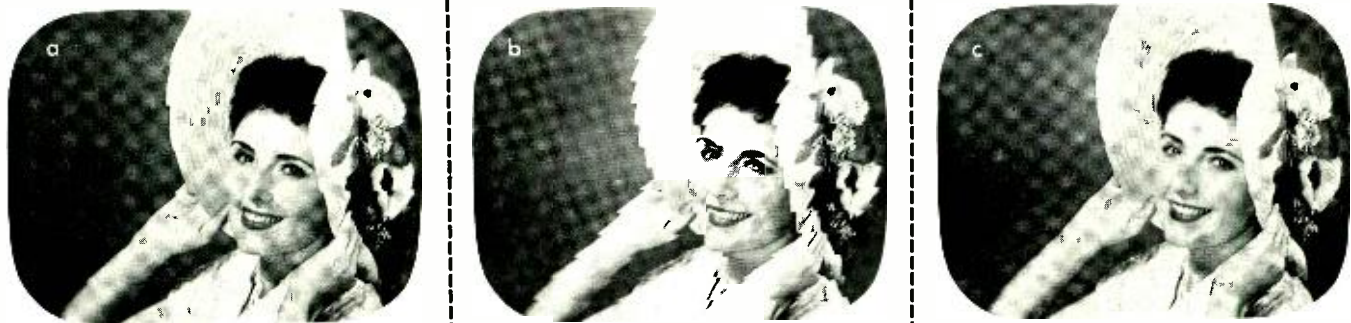
Fig. 1—Three photos from the picture monitor showing scene material with a) quadrature, b) skewing, and c) scalloping distortions.
