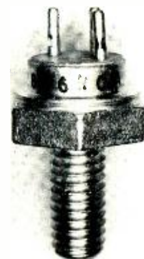
Fig. 3—Over-all package for the 2N2876 transistor.
