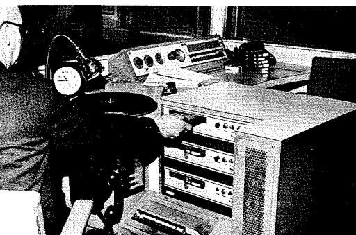
Fig. 5—5C engineer's and director's console. Note convenient position of RT-7 tape machines. Booster amps, intercom, and patch field are located within side and lower sections. Note overseas talkback panel on desk immediately before director's selector panel. The 5C studio is located at upper left.
