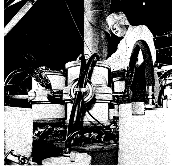
Fig. 6—RCA engineer Nils Oman and part of the largest electronic power supply of its type ever built—an assembly of 500-kw super-power tubes for the C Stellarator fusion-research facility. These tubes supply RF pulses to raise the deuterium in the Stellarator to some 1,000,000°C by ohmic heating process. During the period covered by this article, a joint RCA-Allis Chalmers project, called C Stellarator Associates, designed and constructed the massive C Stellarator facility for Princeton University, who will utilize it in major research on controlled thermonuclear fusion. Engineers and scientists from several RCA Divisions participated in this project.
