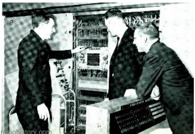
Fig. 2—Trainees shown working on high-speed memory alignment of the RCA 301 during a Training Laboratory session: l. to r. are Instructor, W. Harrison, Kurt Koster and Jim O'Brien.
