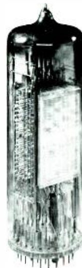
Fig. 3—Selectron memory tube, 256 bits.
