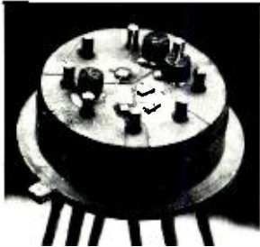
Fig. 1—Ceramic-glass configuration, 0.36 inch diameter.
