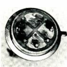
Fig. 2—Ceramic configuration, 0.36 inch diameter.
