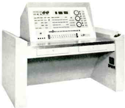
An ATLAS E-series unitary launch-control console.
