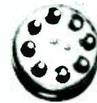
Fig. 10—Multiple-active-device package: a diode transistor gate. Similar examples include a diode gate, isolated transistors, and a Darlington circuit.
