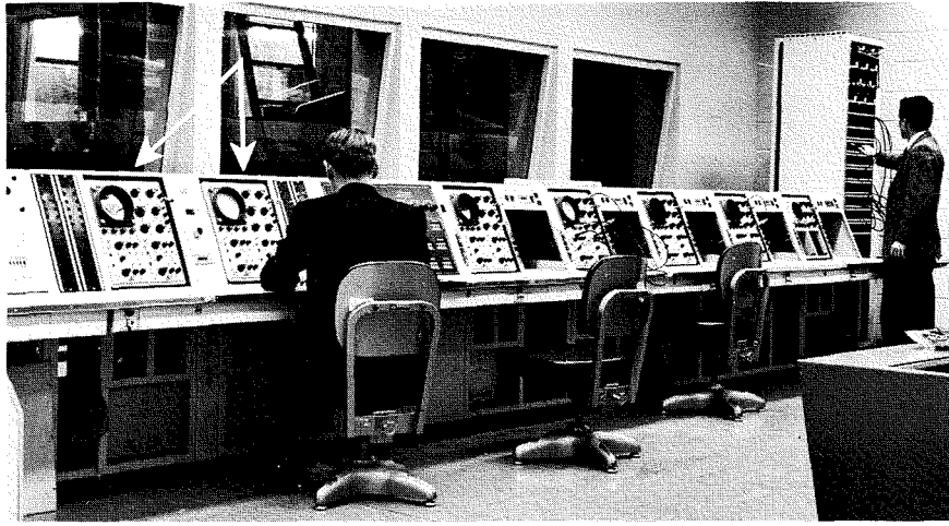
Fig. 1—Present C-Stellarator data system. a. (above) Modular data system consoles in the C-Stellarator central control room. Arrow indicates director's monitoring position. Windows behind the consoles overlook the C-Stellarator itself (see front cover, extreme right). b. (left) Data timer control console. c. (lower left) Data patch board. d. (above, right) TV system monitoring console, also located in the central control room.
