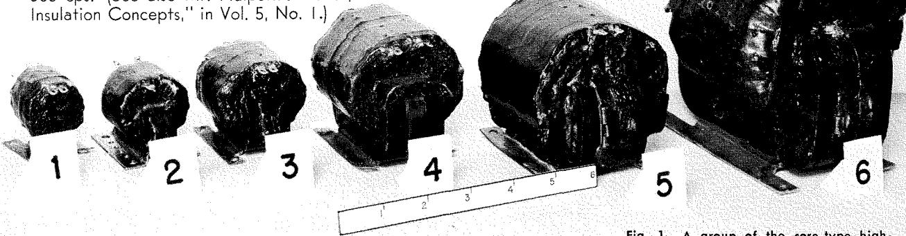
Fig. 1—A group of the core-type high-temperature prototype transformers used in the rating tests and evaluation program.
