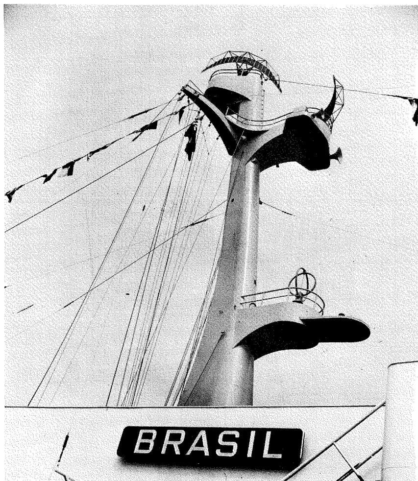
Fig. 3—View of the Radar Antennas and Direction Finder Loop installed on the liner, "Brasil."
