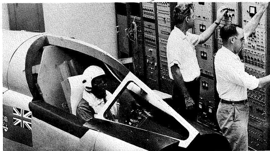
Fig. 3—Human operator tests with cockpit simulator.
