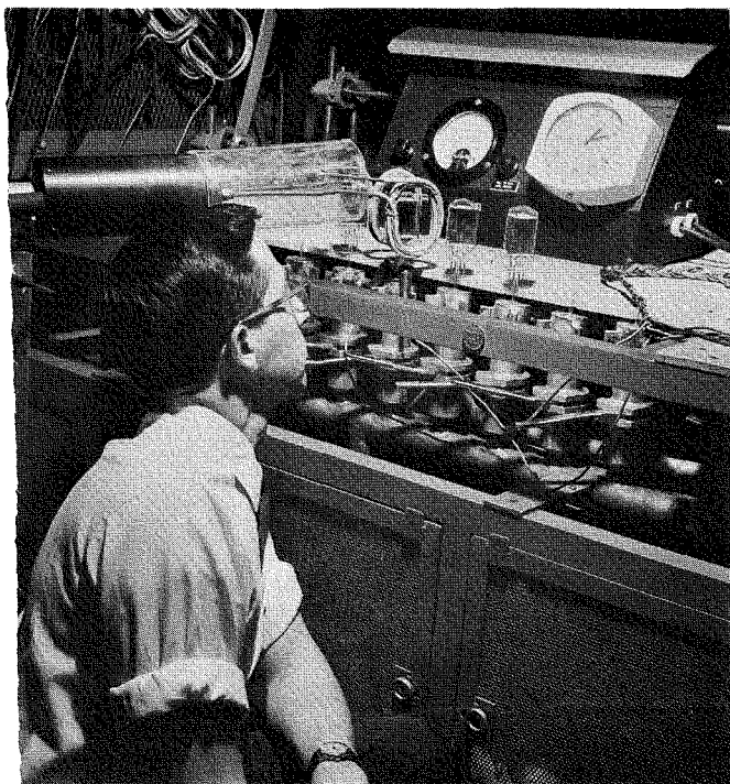
Gil Wolfe, an Engineering Leader, Product Development in the Methods and Process Laboratory, studying the effects of high-frequency heating of the internal parts of a developmental receiving tube while the tube is being evacuated. (Mr. Wolfe has recently been promoted to Manager, Engineering Standards).
