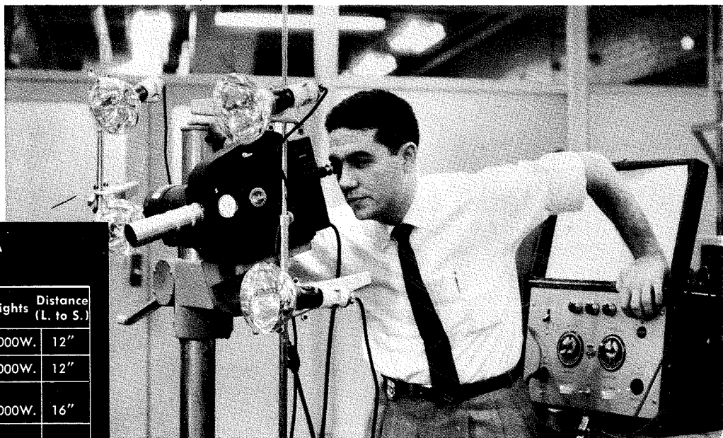
Fig. 1—The high-speed motion picture camera in use. The auxiliary timer-synchronizer unit designed by RCA is shown behind the operator, Frank Marmorato, Equipment Development Machine designer.
