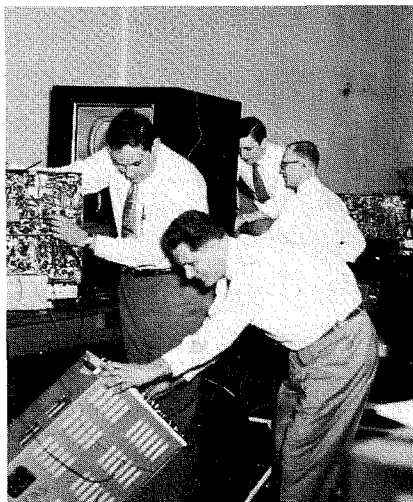
Fig. 3—RCA Service technicians checking matrix on color receivers at the RCA Color Laboratory, Astoria, L.I. Here receivers were prepared for public and industry demonstrations in the New York area.
