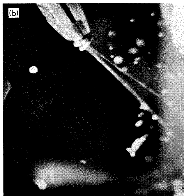
Fig. 5 — Frames from high-speed film of lead-wire tinning machine operation: (a) shows blobs of excess solder thrown off at start of snapping motion; (b) shows thrown-off solder re-landing on lead wires after snapping motion has stopped.
