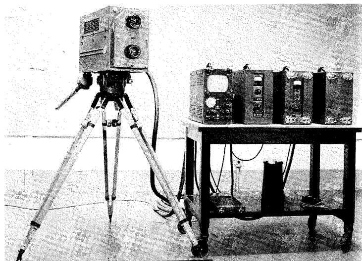
Fig. 11—Early portable field equipment employing the type 1840 orthicon in the camera.
