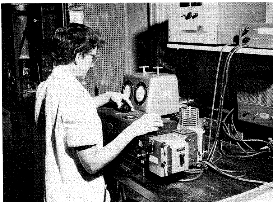
Emma D. Martin performs a spectrophotometric analysis for cyanide in plant processing water before stream disposal. This procedure is calibrated for cyanide concentrations of 0.01 to 0.1 parts per million. Instrumental attachments to the basic spectrophotometer unit include: flame photometer, photomultiplier unit, ultraviolet absorption accessory, and ultraviolet fluorescence equipment.
