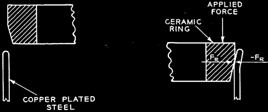
Fig. 4—A radial compression seal
