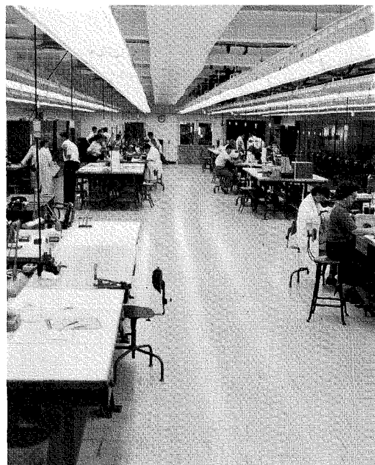
A view of the super-power tube assembly area, called the "white room." Temperature, humidity and dust are carefully controlled to insure constant conditions for tube assembly.
