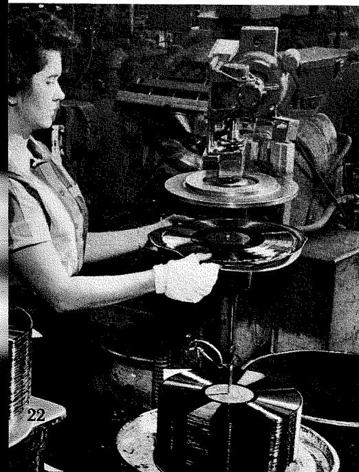
Fig. 3—The operator is placing a freshly molded record in the Hot Knife Edger, which will trim off the excess plastic and produce a smooth finished edge.
