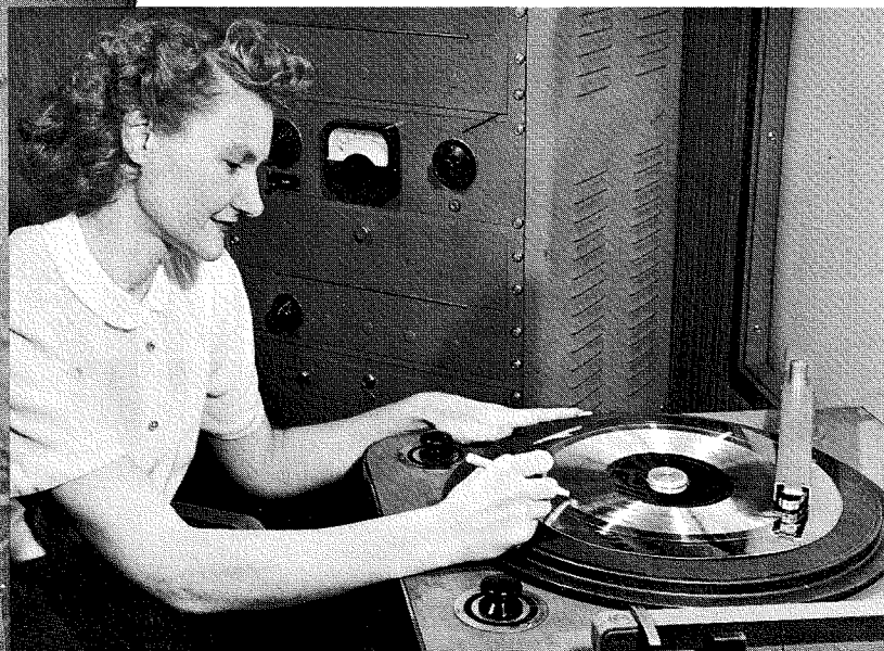
Fig. 6—Play Testing the Mold—The Mold is checked for audio quality.
