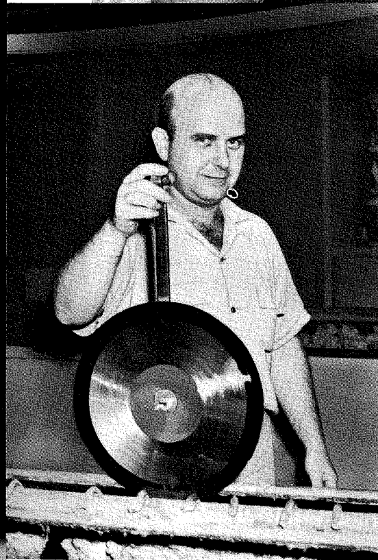
Fig. 3—Nickel Preplate Tank—The silvered lacquer is plated with a layer of nickel .0005 inches thick in this preplating tank.
