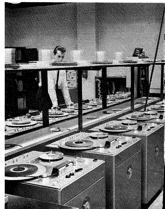
Fig. 4—High-speed tape transfer room.
