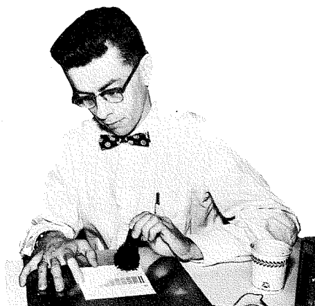
Development of electric-charge image in Electrofax process is demonstrated by H. G. Reuter, Jr., Leader of Electrofax Printer Development. Process was invented by scientists at RCA Laboratories, Princeton, permits rapid making of photographic enlargements without expense of silver-halide light-sensitive coatings on paper.
