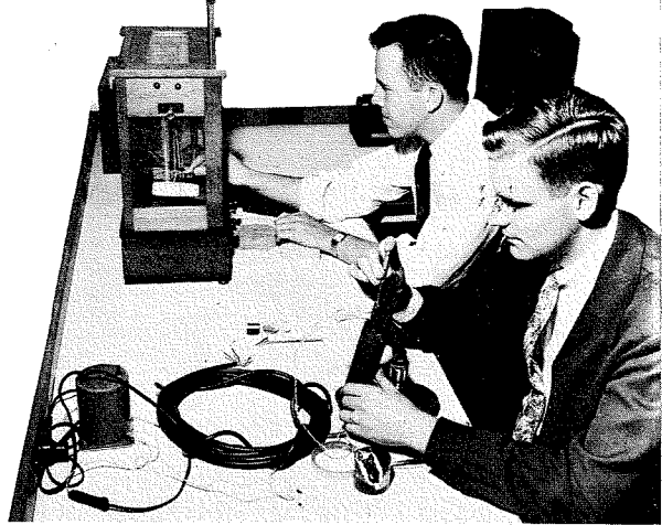
Fig. 5—E. R. Ware (technician in background) and J. W. O'Neill, acoustical engineer shown in the dust-free, transducer design laboratory. Mr. O'Neill is assembling a BK-5A microphone and Mr. Ware is weighing a sample of headphone earcushion material.
