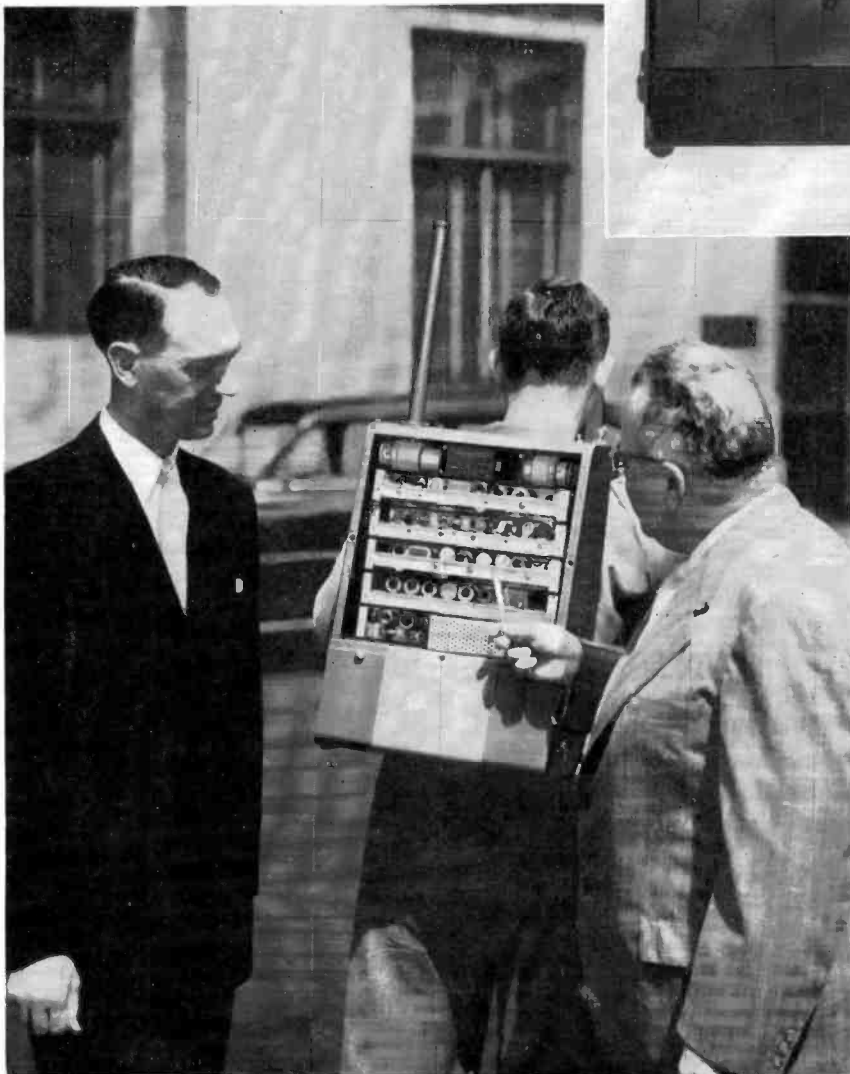
FIG. 10. Closeup of the "Walkie-Lookie" Pack Unit showing the various "plug-in" chassis arrangement used.
