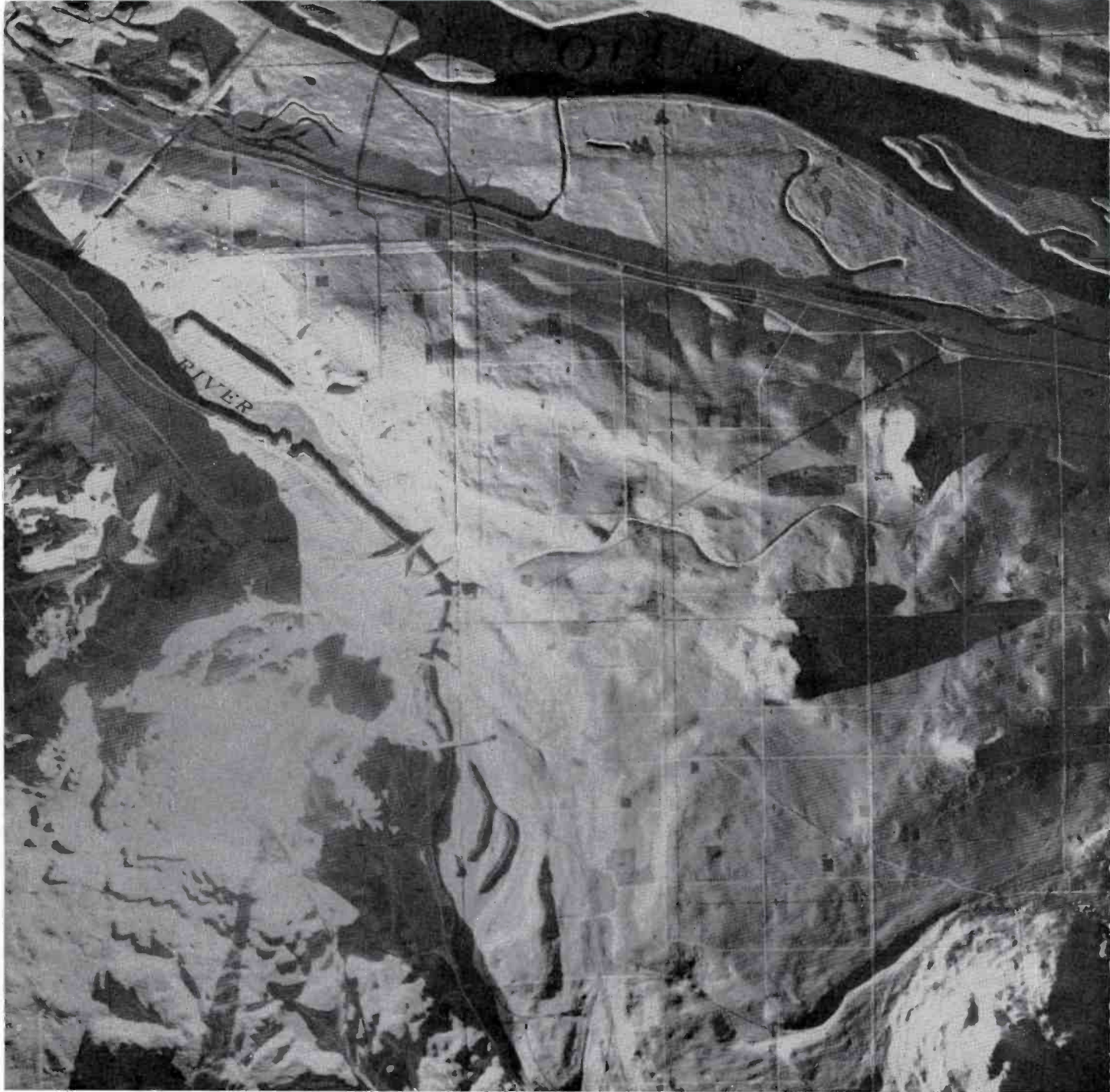
FIG. 13. This "shadowgraph" was made from a relief model in which all of the elevations around Portland were shown on a scale of 500 feet to the inch. A small surgical lamp was placed at the exact position and height of the KPTV antenna. High hills cast shadows which show up plainly in the photograph. The area in this photograph is the same as in the map on the opposite page. It will be noted that the poor reception areas on the map correspond with the shadowed areas in the photo above. However, the UHF reception "shadows" are only about one half as long as the light shadows.
