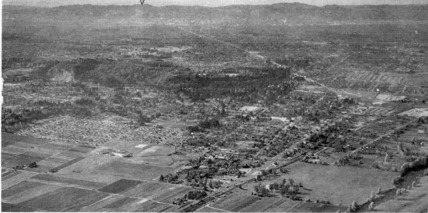
FIG. 16. This is an aerial view of the Portland area from a point about ten miles northeast of the business district. The location of the KPTV transmitter on a 1000-foot ridge on the other side of the city is indicated by the arrow. In the foreground of this picture is Rocky Butte, a sharp-sided hill some 300 feet high which causes the shadow "E" on the map of Fig. 11.
