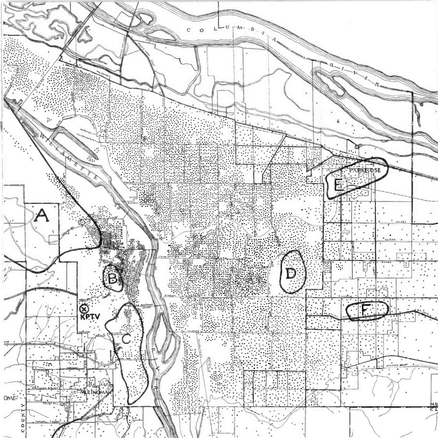
FIG. 14. This is a "population distribution" map of the city of Portland. Each dot represents 40 people according to the 1950 census. "A", "B", "C", "D", "E" and "F" are the areas of poor or no reception, as determined by the method outlined on Pg. 13. By counting the dots in each of these areas it was possible to determine the percent population which will not be able to get good reception at the present time. With later increase in the power of the transmitter, and likely improvements in receivers, the size of these areas will be substantially reduced.
