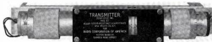
FIG. 9. View of the cavity oscillator or transmitter used in the "Walkie-Lookie" Pack Unit.
