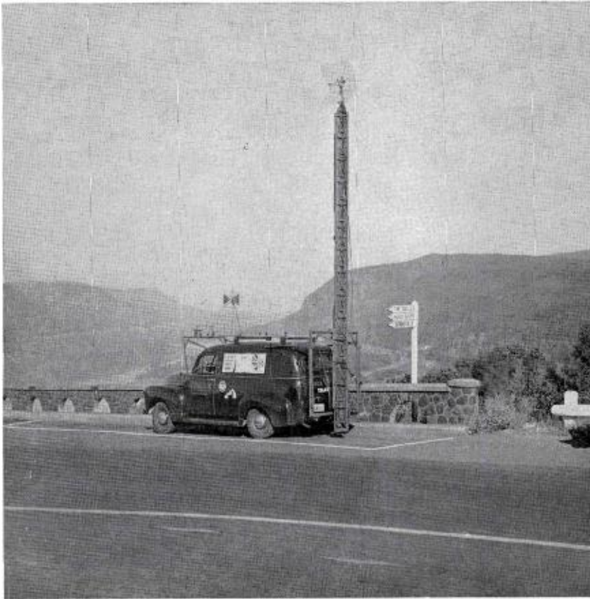
FIG. 5 (left). This is the RCA Service Company's field truck which was used in making the observations on which this report is based. The antenna on the extension tower can be raised to any desired height between 20 feet and 70 feet. For field intensity measurements this antenna was connected to a Stoddard Field Intensity Meter mounted at the observer's position in the truck. The bow tie antenna near the front of the truck was connected to an RCA U-70 Selector feeding into an RCA 630 TV Receiver. Both receiver and field intensity meter were supplied 110 volt power by a small gas engine generator in the truck and could be operated with the truck in motion. The equipment for this field truck was planned and installed by J. D. Callaghan and A. I. Kothe of the Engineering Section of the RCA Service Company. The truck is a part of the permanent equipment of the RCA Service Company's Portland branch. It will be used by technicians in determining the best locations for difficult antenna installations.
