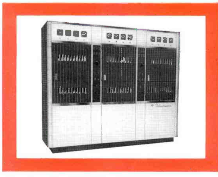
1-KW TYPE TTU-1B (FOR ERP* TO 27 KW). This transmitter and a UHF Pylon Antenna, can develop from 24 to 27 kw ERP on any channel, 14 to 83. TTU-1B is self-contained and all air-cooled. It is well suited as a driver for a high-power amplifier.
