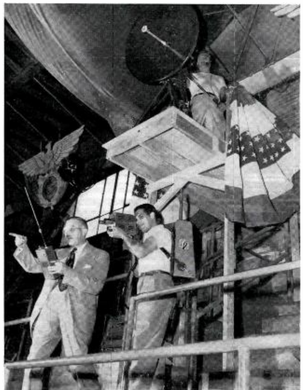
FIG. 2. Another "action shot" taken at the Republican National Political Convention in Chicago. Note the microwave equipment shown mounted on a platform above the "Walkie-Lookie" Unit.
