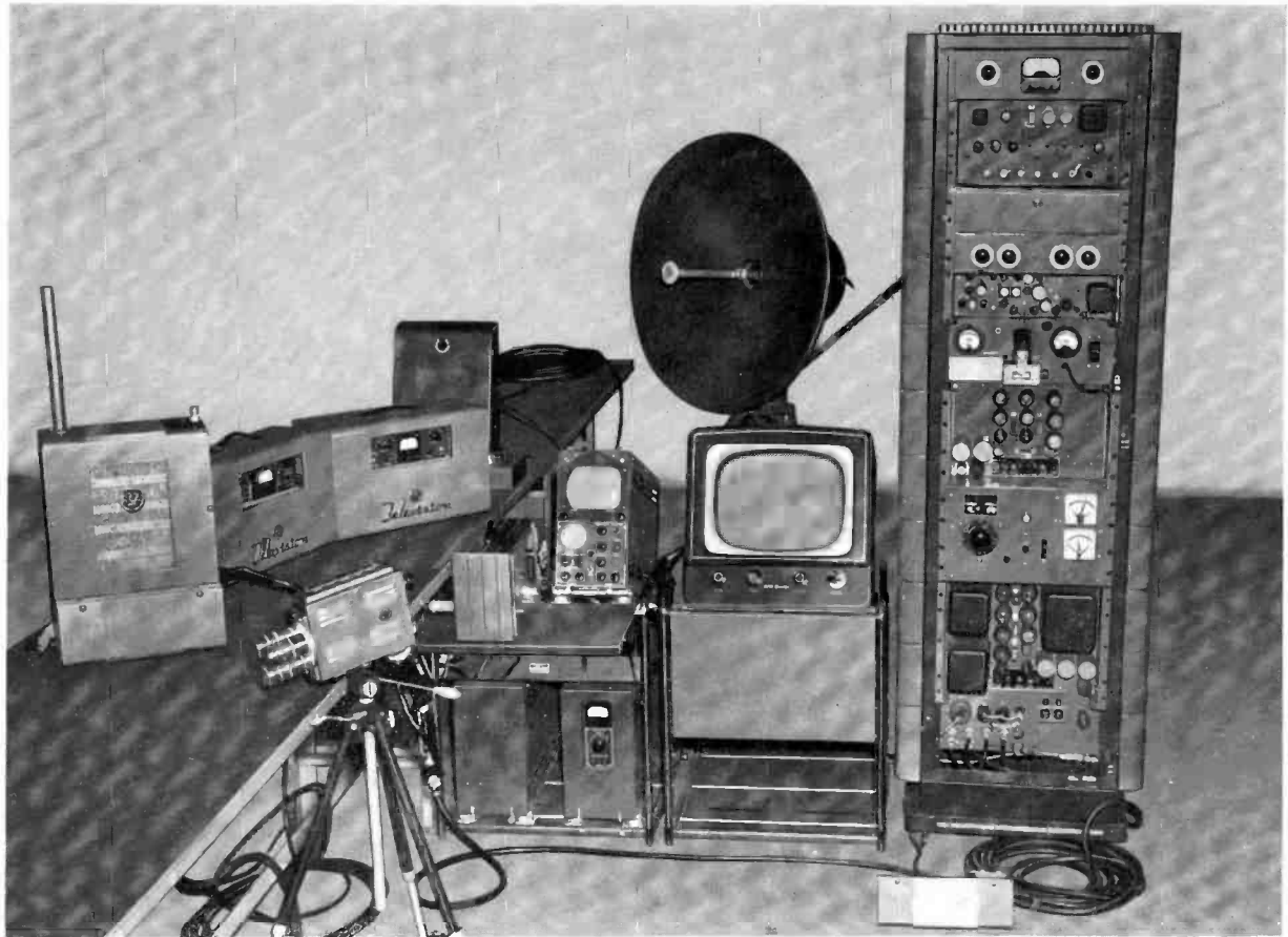
FIG. 14. View of the overall equipment which comprises a complete "Walkie-Lookie" system.
