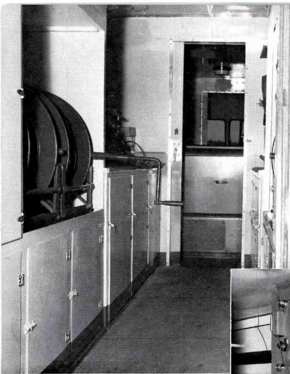
VIEW through the rear doorway of the transmitting power vehicle. Cable reels at left (and right) of corridor are for storing camera cables and power cables. Repair benches can be seen forward of the reels, and one of the gas-engine generators is visible in the next compartment behind the driver's compartment.
