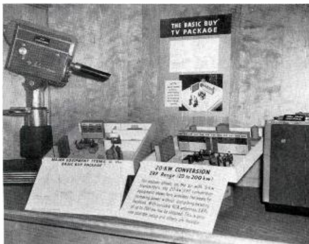
Display of the RCA "Basic Buy" for television broadcasters and 20-kw conversion equipment which enables 5-KW stations to obtain up to 200 kw (ERP).
