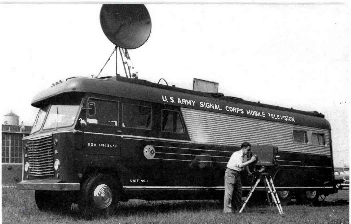
Technical facilities to provide a complete, self-powered TV system, from cameras to receivers, are contained in four six-wheel coaches like the one shown above.
