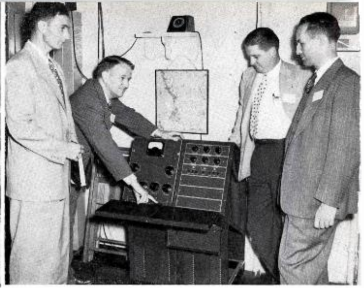
J. Roe, RCA Television Engineer, describing new TC-4A Audio/Video Console which makes possible simultaneous switching. Unit is used to form part of RCA's "Basic Buy" Package for Television.
