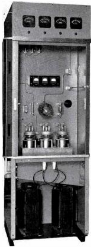
FIG. 18. Front view of power amplifier unit showing 5782 tubes.
