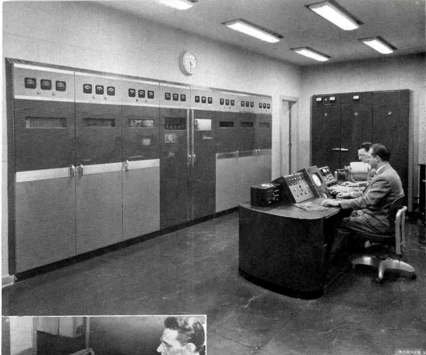
FIG. 1. Transmitter room of WDAF-TV showing built-in RCA TT-5A. Seated at transmitter console are Mr. Byron A. Carlisle and Mr. Stewart Williams, WDAF-TV engineers. Mr. Carlisle designed the microwave-relay rotating unit shown on another page.
