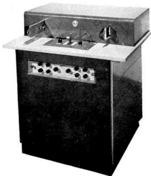
CONSOLE TYPE CABINET houses the complete Flying Spot Scanner and the variable masking arrangement used in obtaining video effects. (Additional circuits of the video effects equipment are mounted in a rack unit which may be located some distance away.) Two slide holders (each holding six slides) may be seen projecting from the upper case at convenient table level. Between them are located fading and lap dissolve controls. The operator can handle all operations from a comfortable sitting position.
