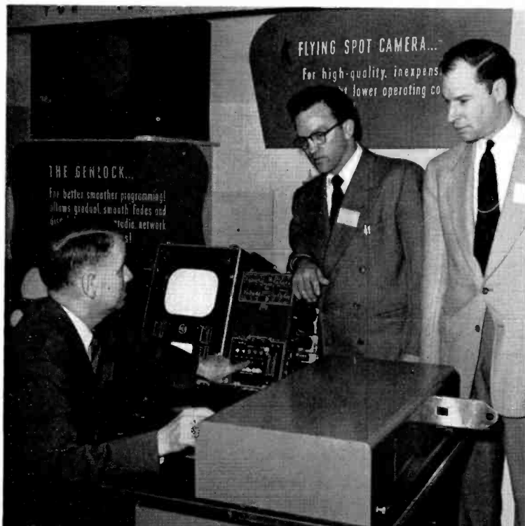
CONVENIENT OPERATION of the Flying Spot Scanner-Video Effects Unit is demonstrated by John H. Roe, Manager of RCA Television System Engineering Group, at the NAB Convention. The console unit may be conveniently placed near the studio control equipment, as shown here.
