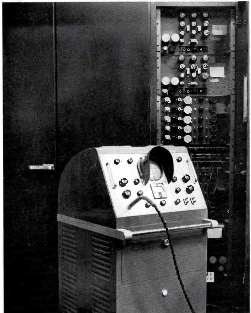
FIG. 3. In order to accurately reproduce these waveforms the oscilloscope used must have a response of at least ten times the horizontal pulse frequency. Either the regular monitor scope (which has a response 300 times the pulse frequency) or an RCA 715-B Oscilloscope, such as that shown here, may be used.
