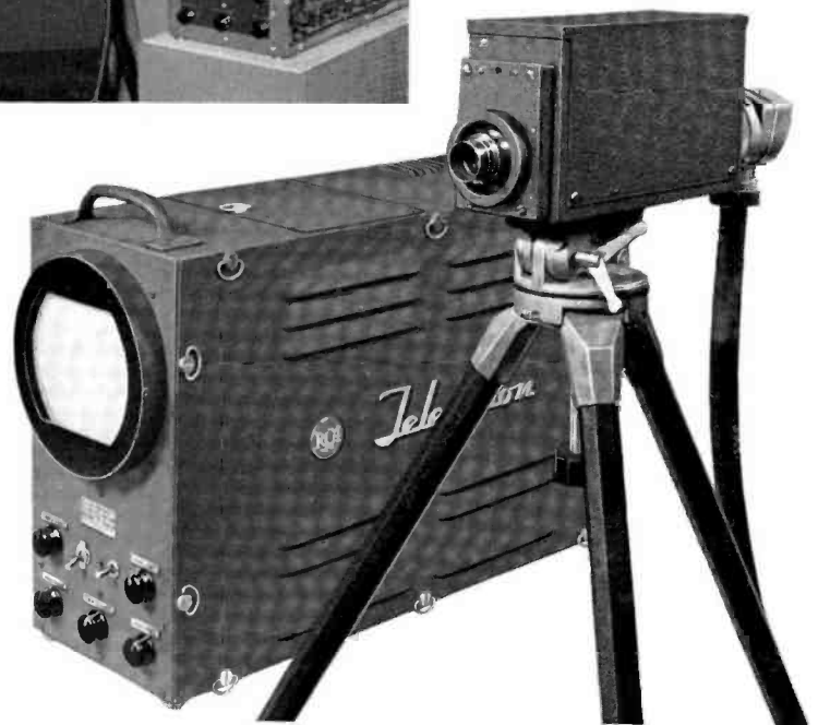
VIDECON EQUIPMENT is complete in these two units. The camera proper is only a little larger than a 16mm movie camera. The control unit which contains the sync generator, deflecting circuits, video amplifiers, controls and monitor kinescope is the same size as one of RCA's standard field units.
