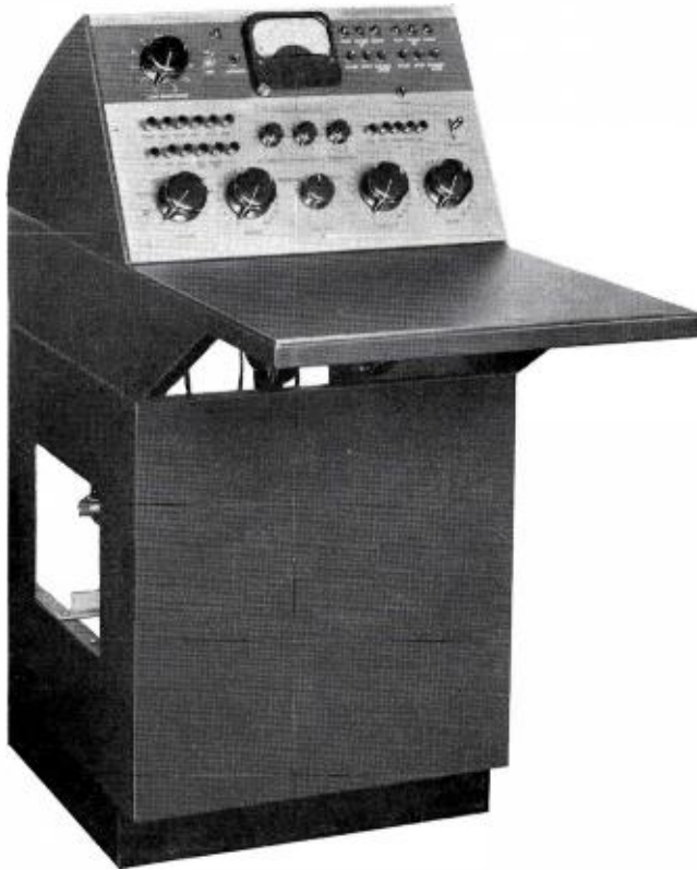
FIG. 4. TTC-3A1 Audio/Video Switching Console consists of a switching turret, desk section and relay/lamp power supply which is mounted in the desk.
