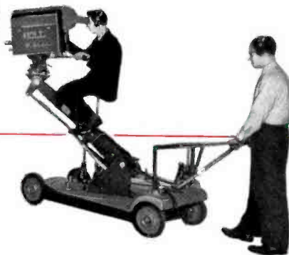
RCA Studio Dolly, Type MI-26040. This crane-type portable dolly enables the camera man to move in and out—add variety to otherwise static scenes. The camera is lowered and raised manually. The entire assembly rotates horizontally around its base. This dolly can be silently transported around the studio while the camera man focuses the scene.
