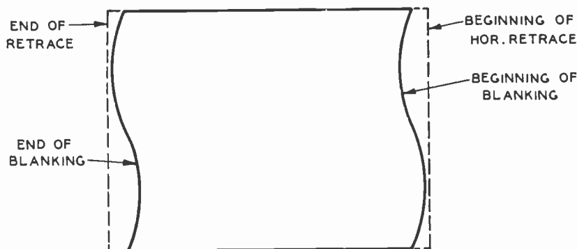
FIG. 10 (right). Effect of frequency modulation of horizontal sync and blanking on shape of raster in receiver with AFC of horizontal scanning.
