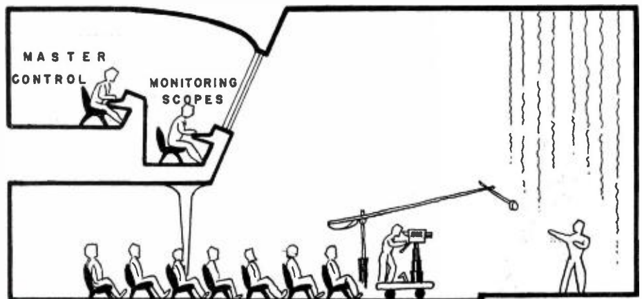
FIG. 2. Section through studio and control room of the studio plan shown in Fig. 3 and Fig. 4 (following pages).
