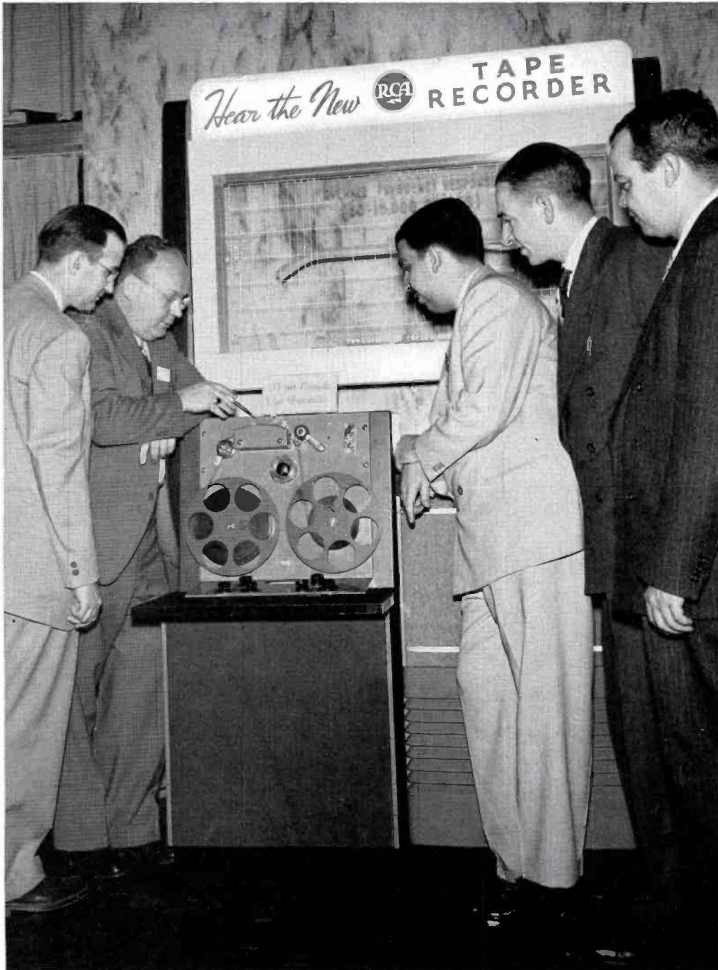
FIG. 1. Ease of threading tape and other features of the plug-in recorder head of the new RCA Tape Recorder, Type RT-4A, are pointed out to broadcasters by M. A. Trainer, Merchandise Manager of RCA Studio Equipment.
