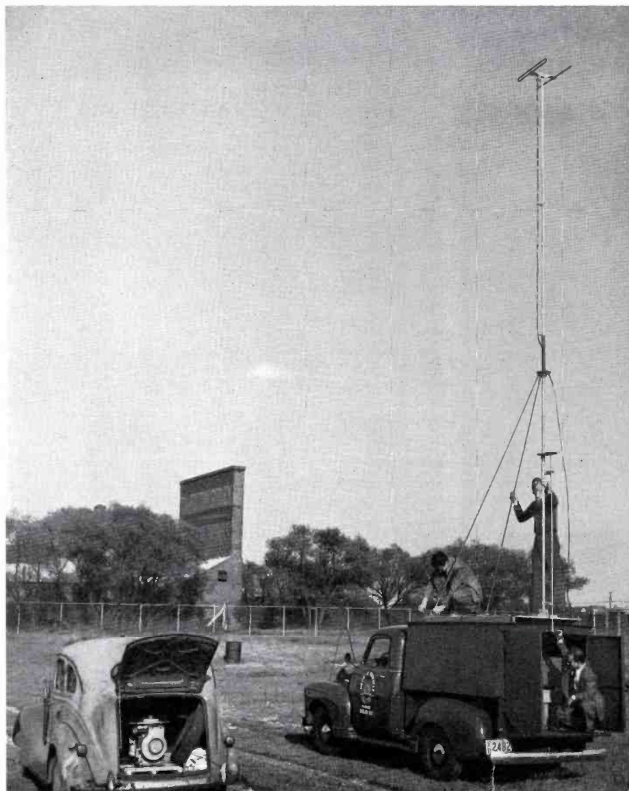
FIG. 2. A 750-watt gasoline powered generator supplied all the power necessary for the receiving and calibrating equipment located in the mobile monitoring truck.
