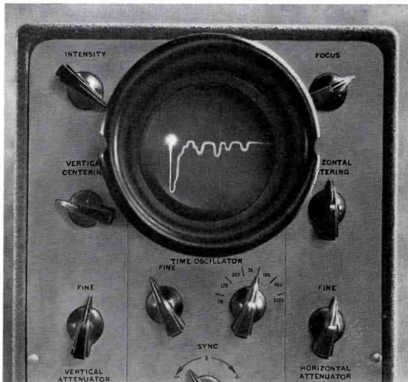
FIG. 10. This photo of the oscilloscope was taken under conditions of severe multi-path reception. The main pulse (negative polarity) is shown directly below the bright dot. Note that first echo occurs during the decay time of the main pulse. This echo alone would account for distorted picture on television receivers in the home.
