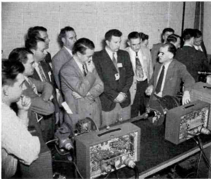
FIG. 7. In the television microwave relay laboratories, C. A. Rosencrans demonstrated the operation of a microwave relay transmitter and receiver by actual functioning units shown on the laboratory table minus the protective weatherproof cans and parabolic "dishes".
