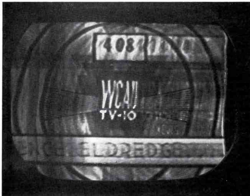
FIG. 11. This photograph of test pattern from television transmitter, also made under specially severe multi-path conditions, was taken at same location as that of Fig. 10. Note correlation between pulse echoes shown on the oscillogram and those shown in this photograph. (For a picture of WCAU-TV's unique "news, time and music" test pattern as received at most locations, see BROADCAST NEWS No. 54, page 52.)
