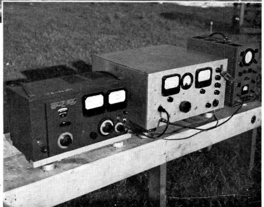
FIG. 5. Shown at right is a closeup of receiving and measuring equipment which was mounted in the truck. From left to right, the units are: the standard signal generator; the modified RCA 8TS30 television receiver; and the Type WO-79B pulse oscilloscope. The RCA 8T241 picture receiver is not shown.
