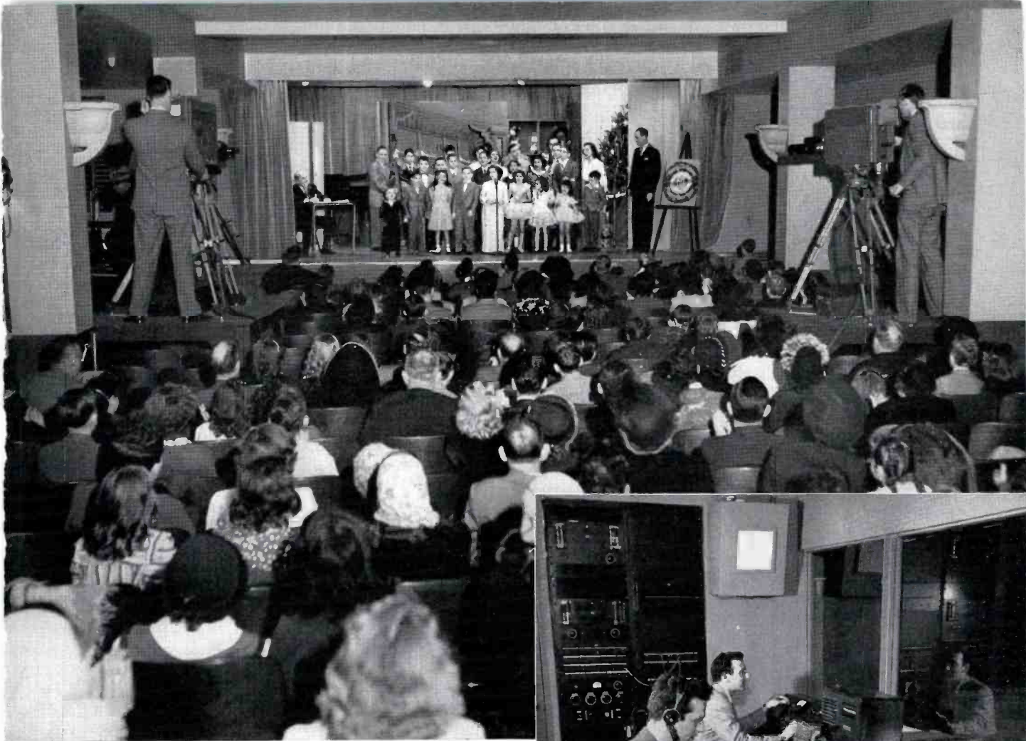
FIG. 10 (above). WCAU-TV's Studio X, shown above, is a 250-seat auditorium on the second floor of the building, designed originally for audience-type radio shows. It was easily modified for television and has worked out very well. Note cameras which are mounted on four-foot wooden platforms, two on the left of the auditorium and one on the right near the center.
