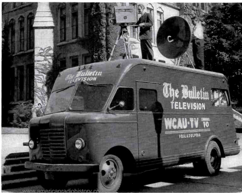
FIG. 32. WCAU-TV's Field Equipment is a standard RCA TJ-50A Mobile Unit furnished with three camera chains, master monitor, relay equipment and accessories.
