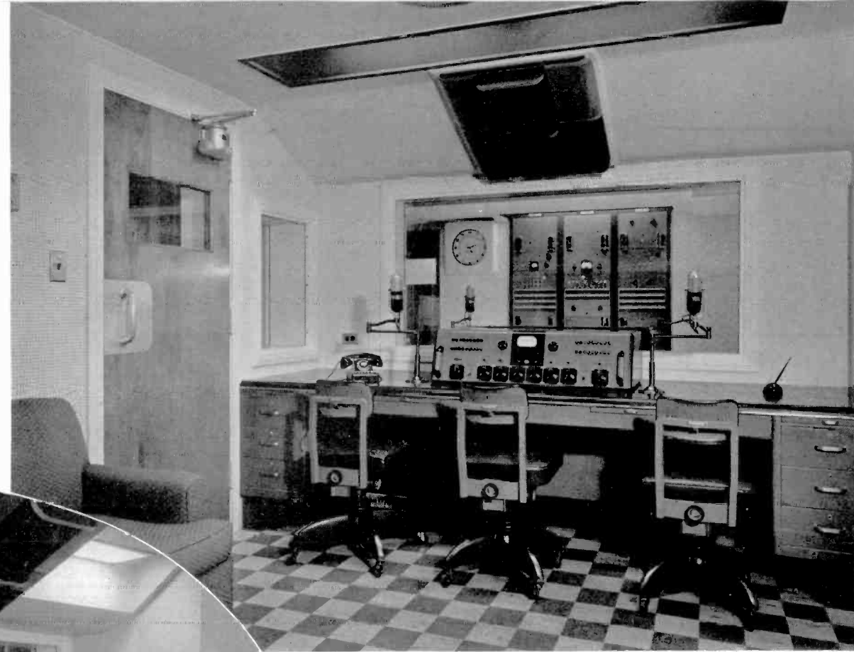
▲ Control Room for Studio B is provided with two announce positions and an RCA 76-B1 Console. The Studio C Control Room and Master Control Racks may be seen through the window. ◀ The WREC Transcription Recording Room is equipped with two RCA 73-A DeLuxe Recorders. Note the RCA 64-B speaker mounted in the ceiling.
