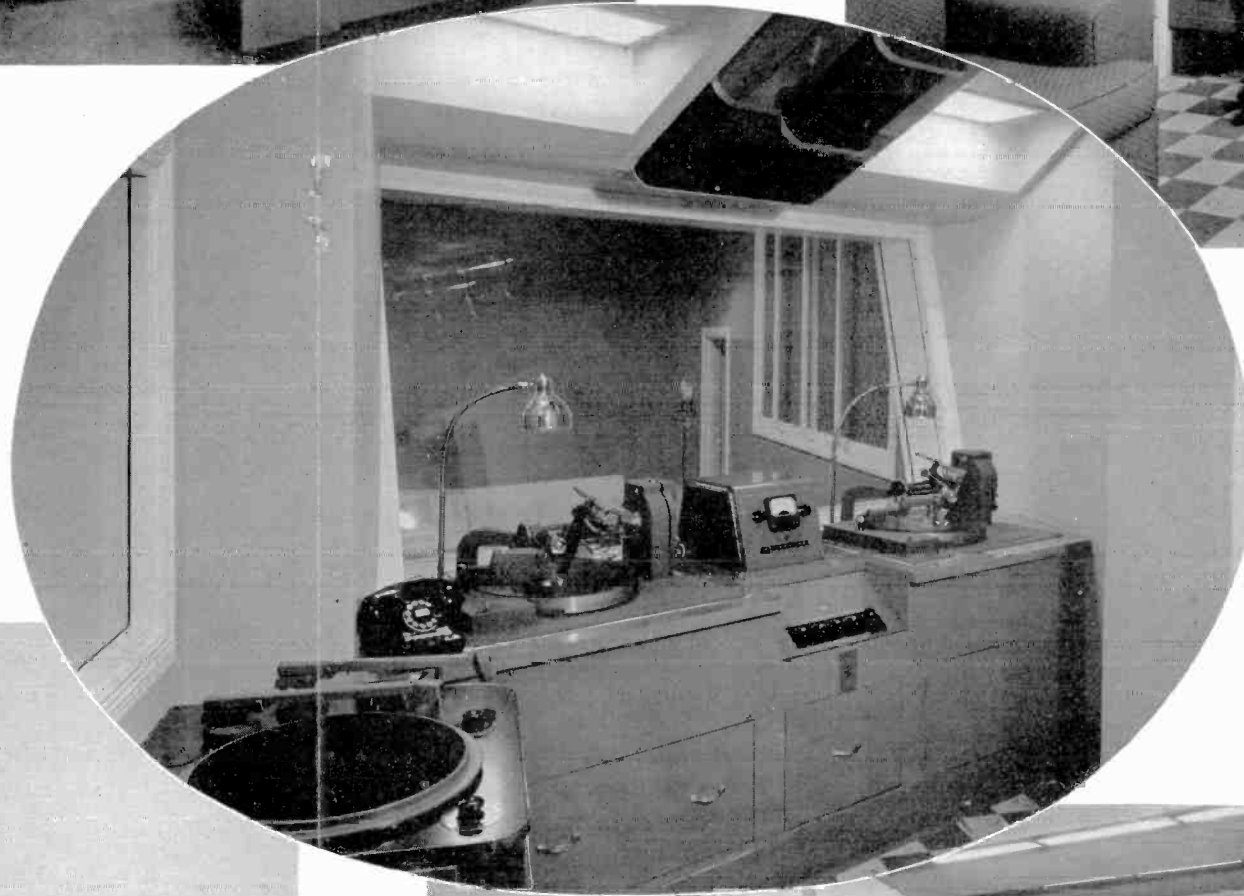
▲ Control Room for Studio B is provided with two announce positions and an RCA 76-B1 Console. The Studio C Control Room and Master Control Racks may be seen through the window. ◀ The WREC Transcription Recording Room is equipped with two RCA 73-A DeLuxe Recorders. Note the RCA 64-B speaker mounted in the ceiling.
