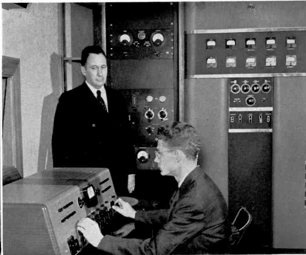
▲ WMCB, Mobile, features the 250 K and 76 B Console in its layout. WMCB was the first 250 K on the air.
