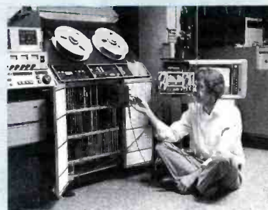
Greg Fox, Video Chief Engineer, maintains the high quality of equipment standards and operation. Here, a TR-600A quadruplex VTR is set-up to facility requirements.
