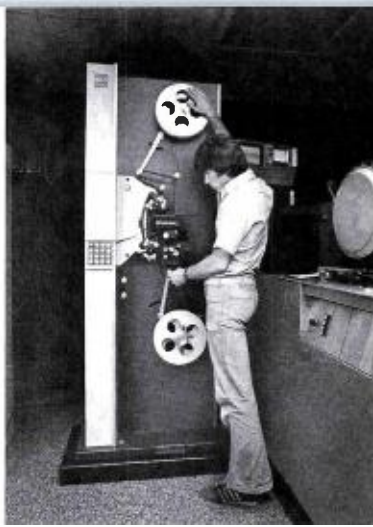
Steve Fraasa loads the RCA FR-35B with negative film to be transferred to three-quarter inch video cassette.
