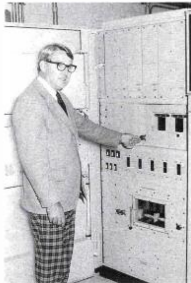
Bernie Moore, Vice President, Engineering at power supply cabinet of TTG-30/30H Transmitter. The key interlock system of TTG Series transmitters is an important safety feature for unattended operations such as that at WBTW-TV.
