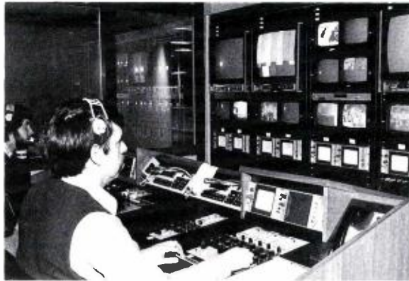
Video control for the two main studios are also identical. Camera controls for eight TK-47 cameras and two TK-760's are mounted in each of these video control consoles.
