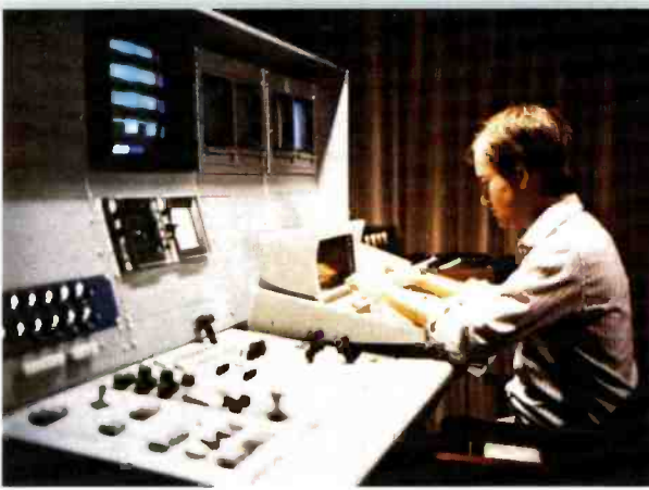
Rusty Hancock, Video Base Vice President, takes an active role in production. The RCA-supplied Datatron Tempo 76 Time Code Editor is employed here during a post production session.
