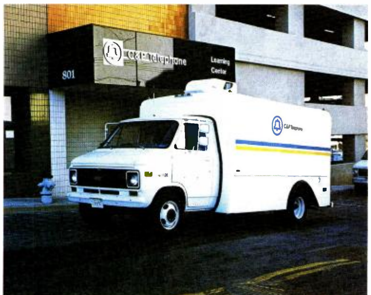
Mobile unit for the Audio Visual Center looks like a C&P Telephone operations vehicle, but carries a complement of equipment for TV production: TK-76 camera; 3/4-inch VTR; audio; lighting.
