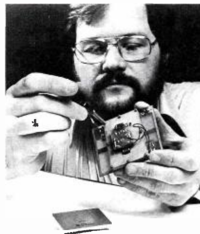
TINY TV FILTER — Technician Kenneth Alderson prepares circuitry for installation of a high precision SAW (Surface Acoustic Wave) filter used in RCA's new "G" line transmitters. The filter (foreground) replaces components weighing more than 500 pounds in older model transmitters, and is used to shape and control visual response for enhanced picture quality.
