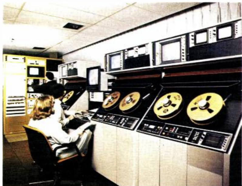
Quad tape editing system includes three TR-600A VTR's with AE-600 Time Code Editing System.
