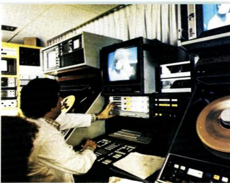
From editing console, operator can edit quad tape, insert material from 8-track audio system and all video and film sources.
