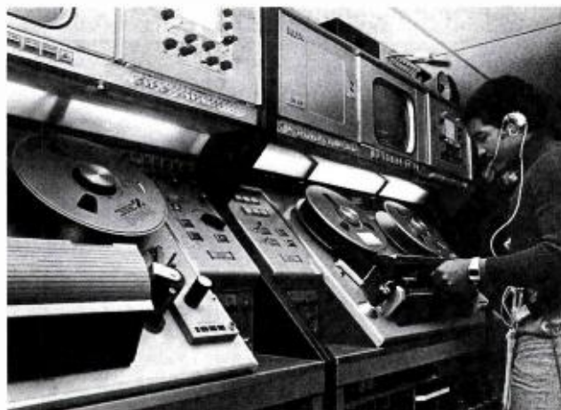
Tape complement for WRAL-TV includes TR-70's and two TCR-100 "cart" machines.
