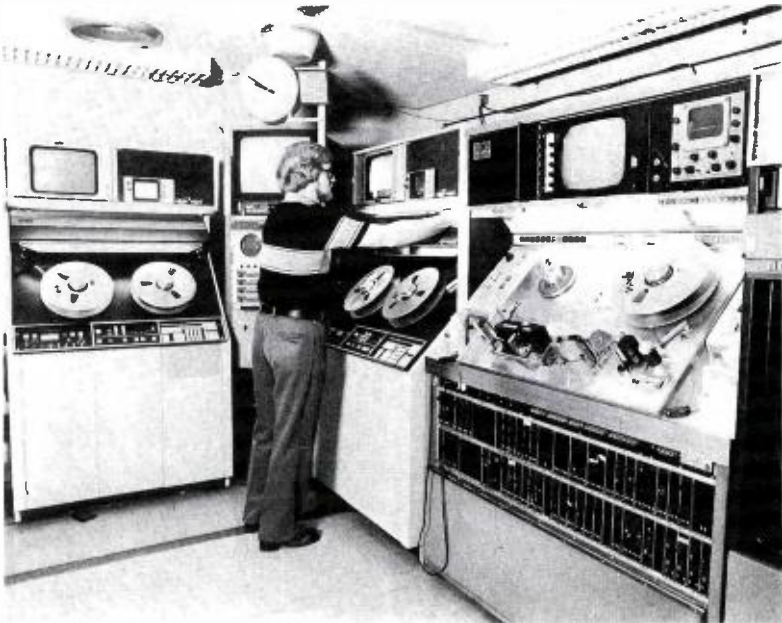
Video tape facilities include two TR-600A quad VTR's with AE-600 Time Code Editing systems. The editing system is being remoted from the tape area to a separate editing suite.
