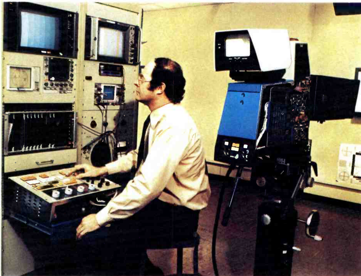
SYSTEMS TEST — A production model of RCA's TK-47 automatic color television studio and field camera is checked out by RCA engineer Frank Davenport during systems test in Camden, N.J. Introduced at the 1978 National Association of Broadcasters convention, the fully-automatic camera features simplicity of operation and microprocessor-
