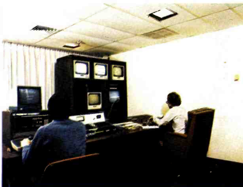
Production control center adjoins studio, with complete facilities for audio and video switching; character generator; camera controls; distribution.
