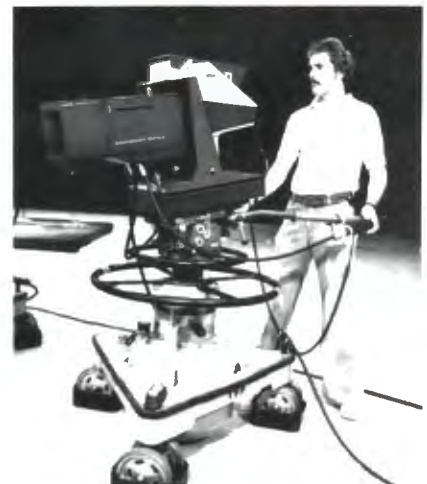
Versatile TKP-45 Production Camera with "Minimax" adaptor is used on location and as a third camera for studio productions.
