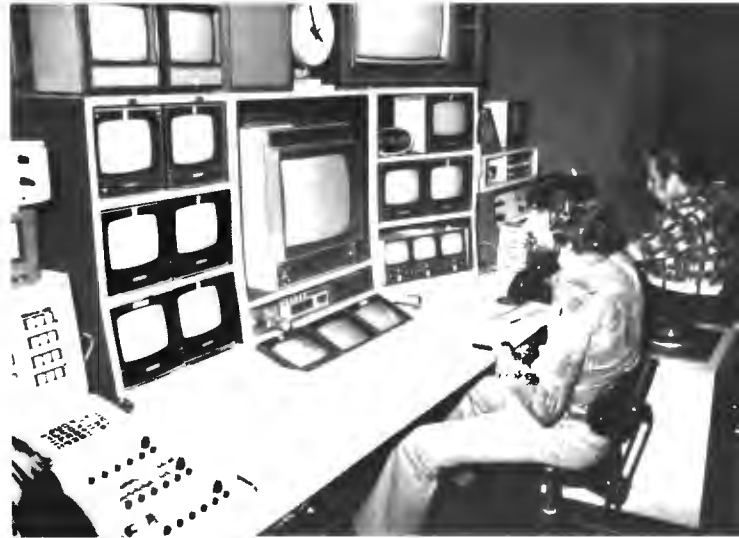
Production Control at TV-11 is a compact, functional layout, with the central TD position flanked by the video switcher (left) and the audio board.
