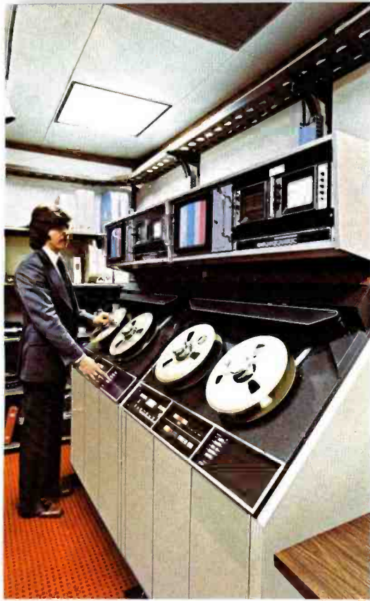
Chief Engineer Pat Howley operates TR-600's in Merrill Lynch video production facility. Quad machines are used for mastering, with edited tapes dubbed to videocassette format for distribution.
