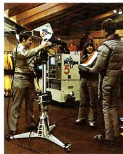
TKP-45 portable color camera used with "Minimote". Its automatic features and light sensitivity make it ideal for indoor and outdoor shoots.
