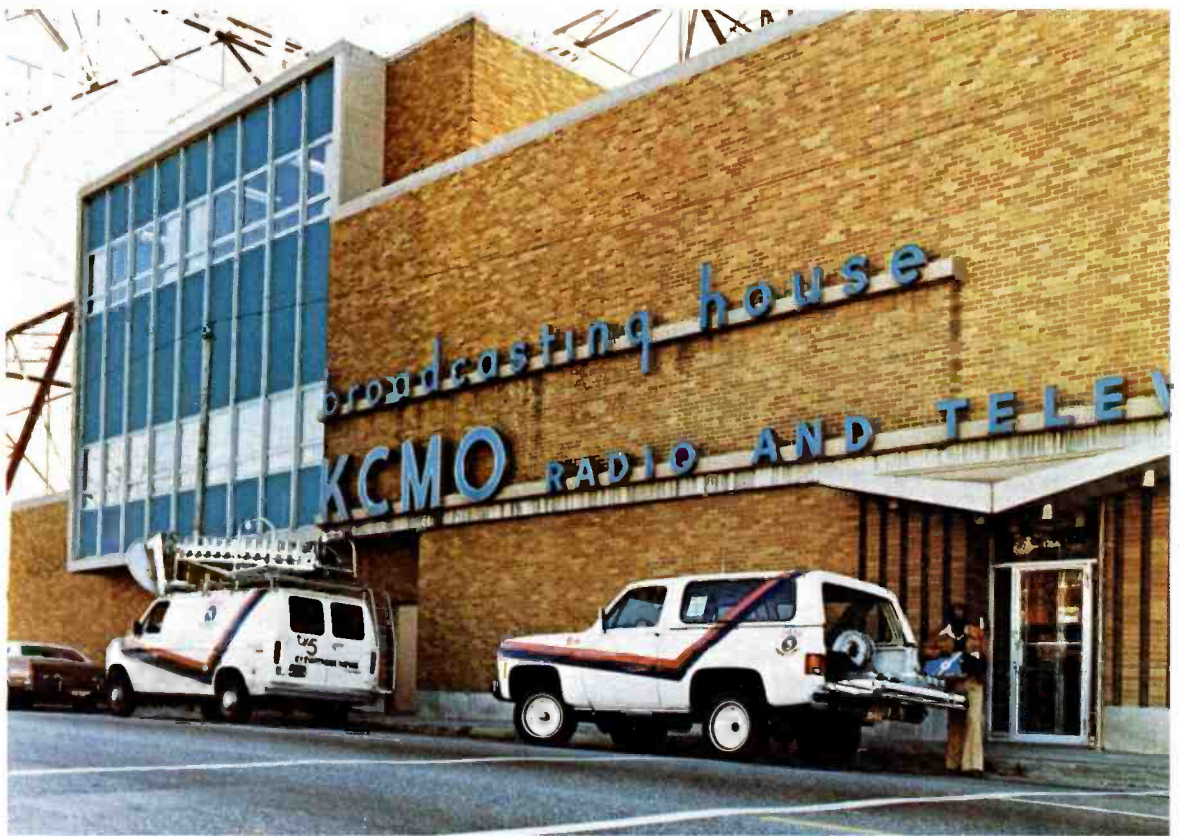
New ENG vehicles in front of KCMO building. Van at left is a Type I or "mother" vehicle, with microwave capability. At right is the Type II reporter vehicle. This ENG system, designed by KCMO engineering, is being adapted for use by all Meredith Broadcasting stations.
