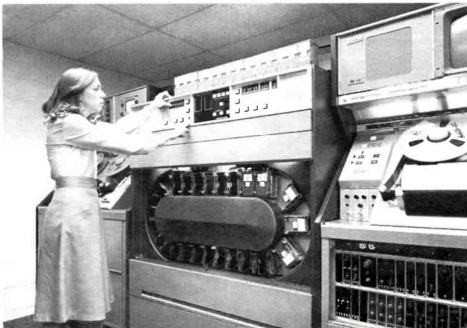
WDCA-TV pioneered use of TCR-100 "cart" machine, with first system installed in 1969. On average, 300 tape "carts" are aired daily.
