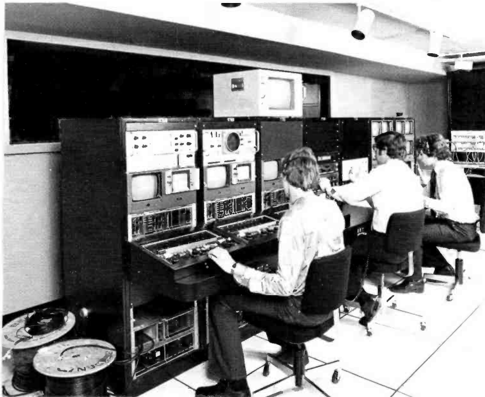
Chief Engineer Pat Howley operates TR-600's in Merrill Lynch video production facility. Quad machines are used for mastering, with edited tapes dubbed to videocassette format for distribution.
