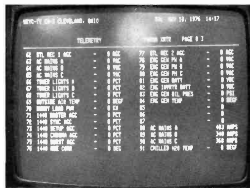
Computer-controlled system provides instant access to programmed transmitting system data. Telemetry, metering and numerous other system operating functions are available for display as "pages" on the video monitor.
