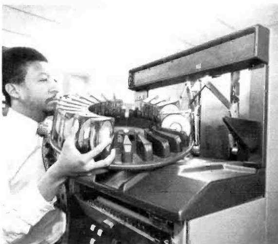
TCP-1624 Film Cartridge Projector system has eased strain on Telecine. Incoming film spots are easy to load in cartridge. Up to 24 "carts" can be loaded on magazine.
