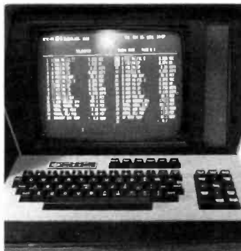
Keyboard and CRT display unit for DCS-2 system located in the transmitter control area.
