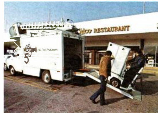
Ramp attached to rear bumper of van permits easy loading and off-loading of "Minimote" cart.
