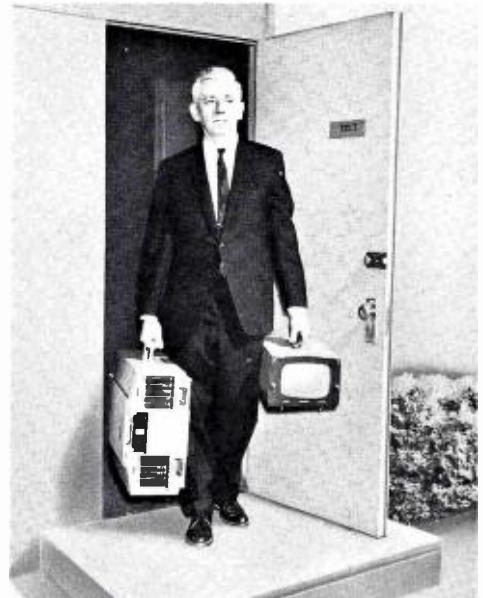
Separate viewfinder and camera units make the TK-33 easy to carry—always ready for remotes.
