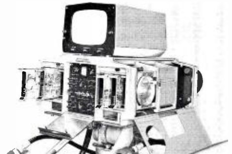
Plug-in transistorized modules, high-brightness 8-inch viewfinder are deluxe features of this new field camera.
