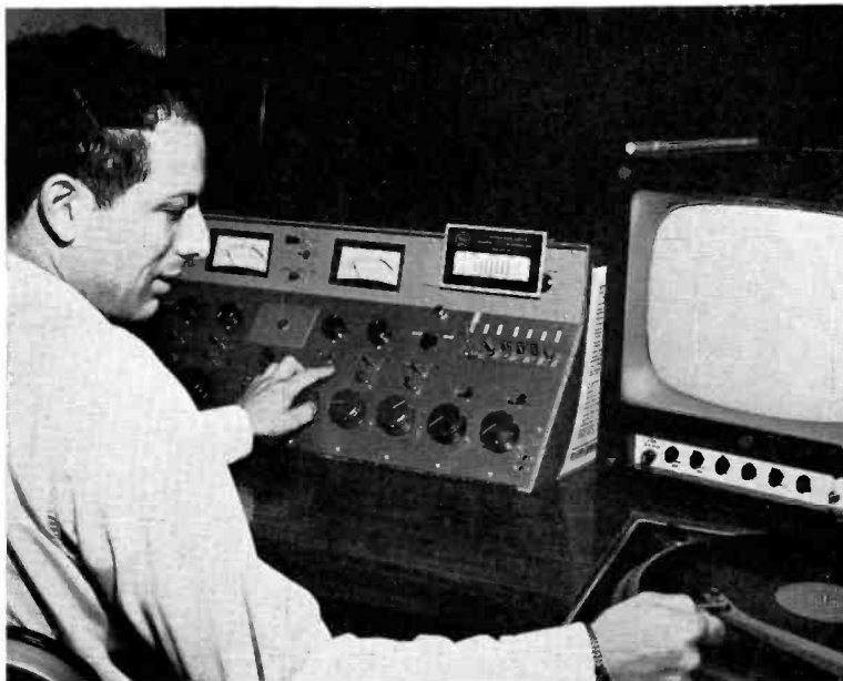
FIG. 6. (above) At the right of the audio position in each of KCET's control rooms there is an RCA BQ-2C Turntable. LC-1A Speakers are mounted above the control room window.
