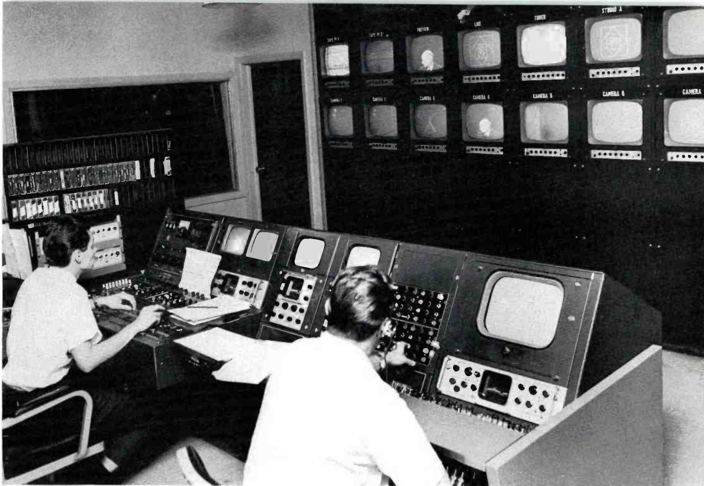
FIG. 8. (above) KCET Master Control includes a master switching position at the far left and film and tape control, right foreground. Monitors in back wall show individual camera outputs as well as studio outputs, tape outputs, line, etc.
