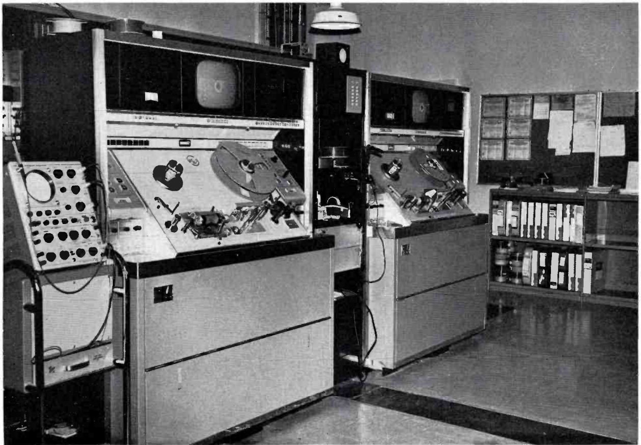
FIG. 11. (below) The other side of the Telecine area showing KCET's two RCA TR-22 Tape Recorders. There is also a TR-4 Tape Recorder and a TR-3 Player.
