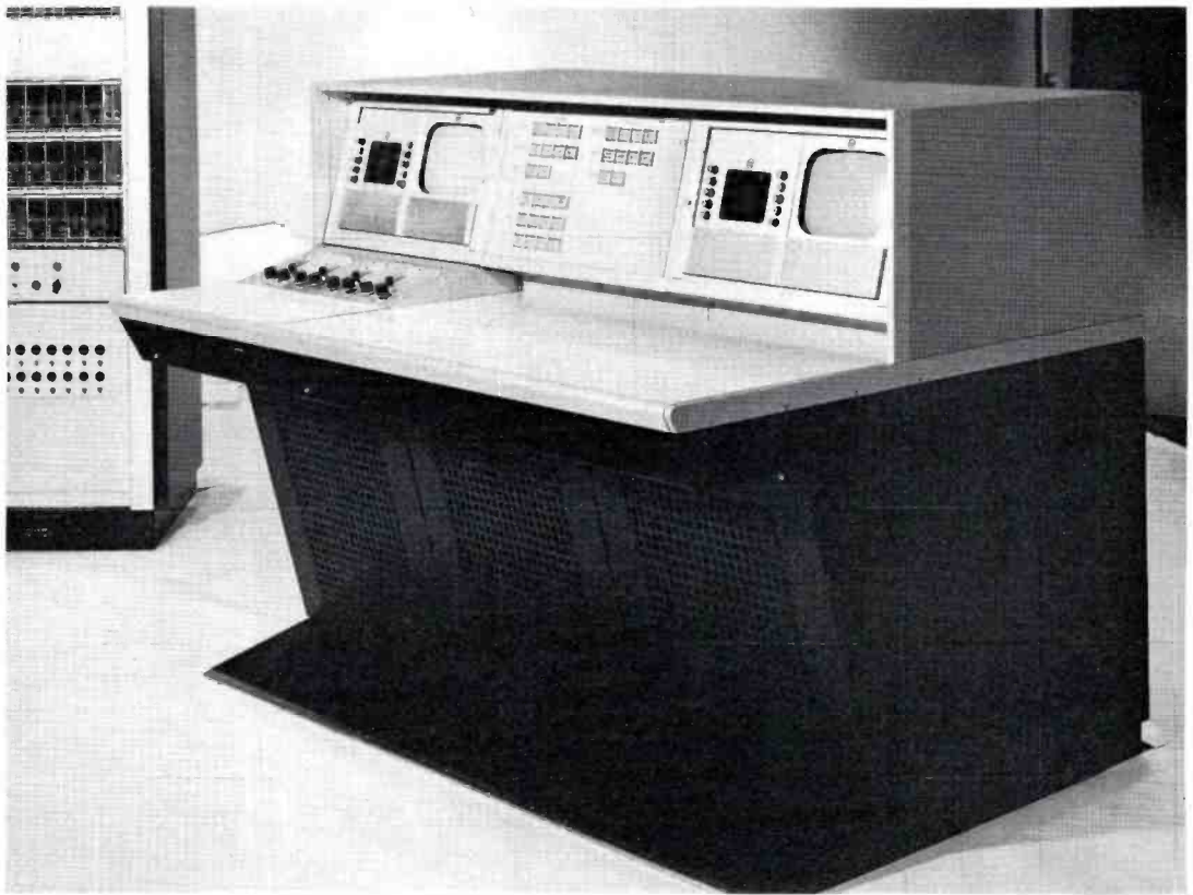
FIG. 10. New-style consoles are made up of modules which can be assembled to fit any requirement. Left section of this 3-section console contains picture and waveform monitors and controls for four monochrome cameras.
