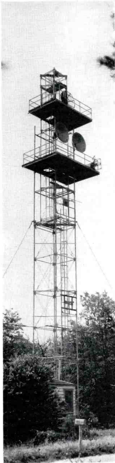
◀ FIG. 4. During antenna-pattern tests, radio energy is beamed at the antenna from this tower almost three miles east of the test site. The 100-ft. tower supports several antennas.
