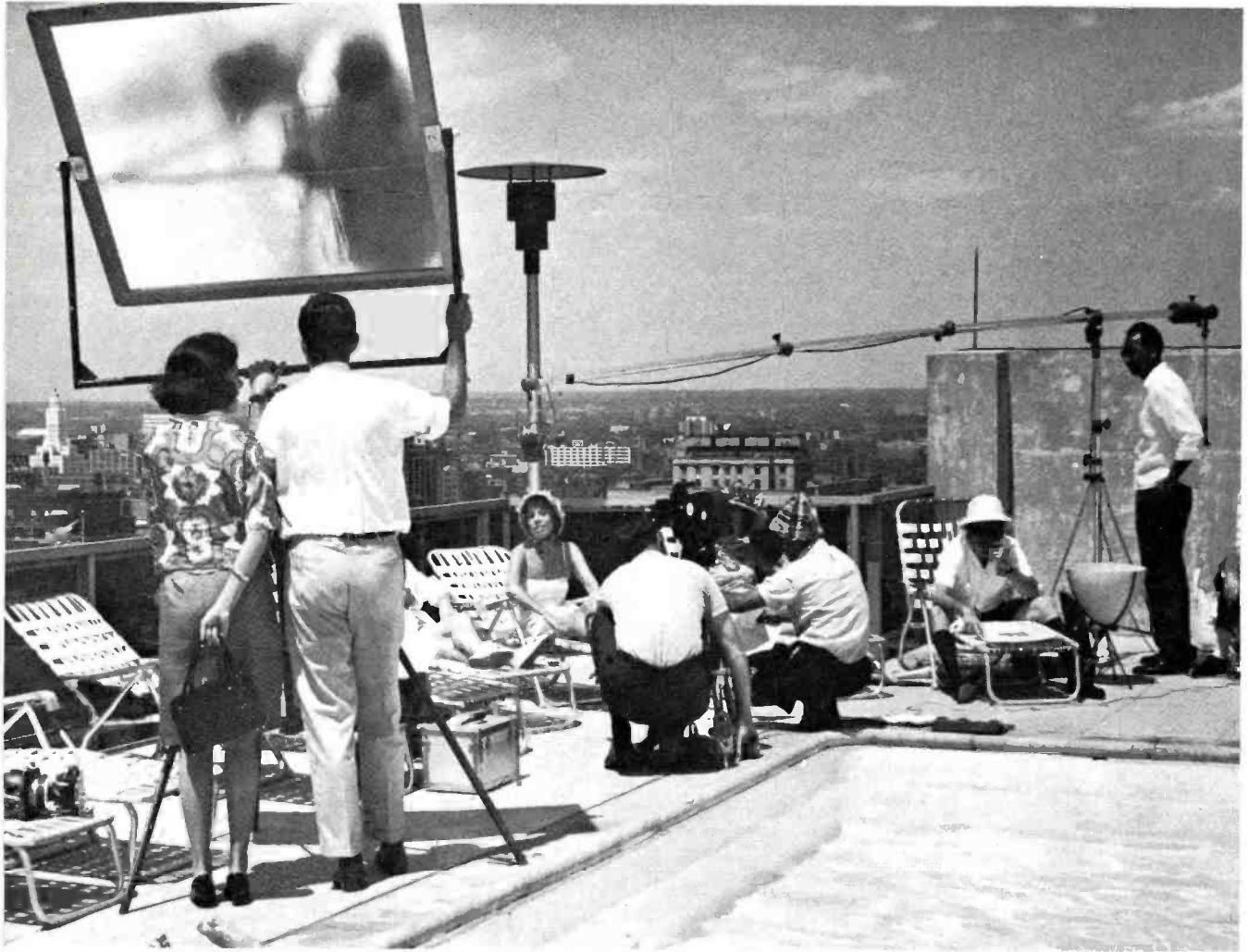
FIG. 7. WCAU-TV film crew at work on a scene in current color production. Note use of giant reflectors. These assist in keeping uniform color temperature, assuring color fidelity.
