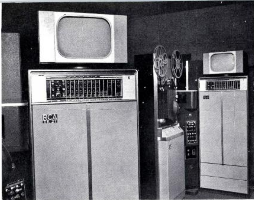
FIG. 1. WCAU-TV has installed two of the New Look RCA 4-channel color film chains Type TK-27, complete with TP-15 Multiplexers, TP-66 Film Projectors and TP-7 Slide Projectors.
