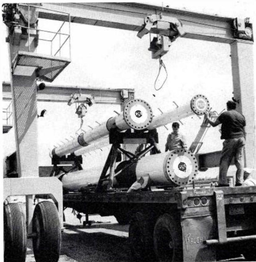
FIG. 19. This photo shows the last stages in loading a traveling-wave antenna aboard the flatbed truck that takes it to its new owner.
