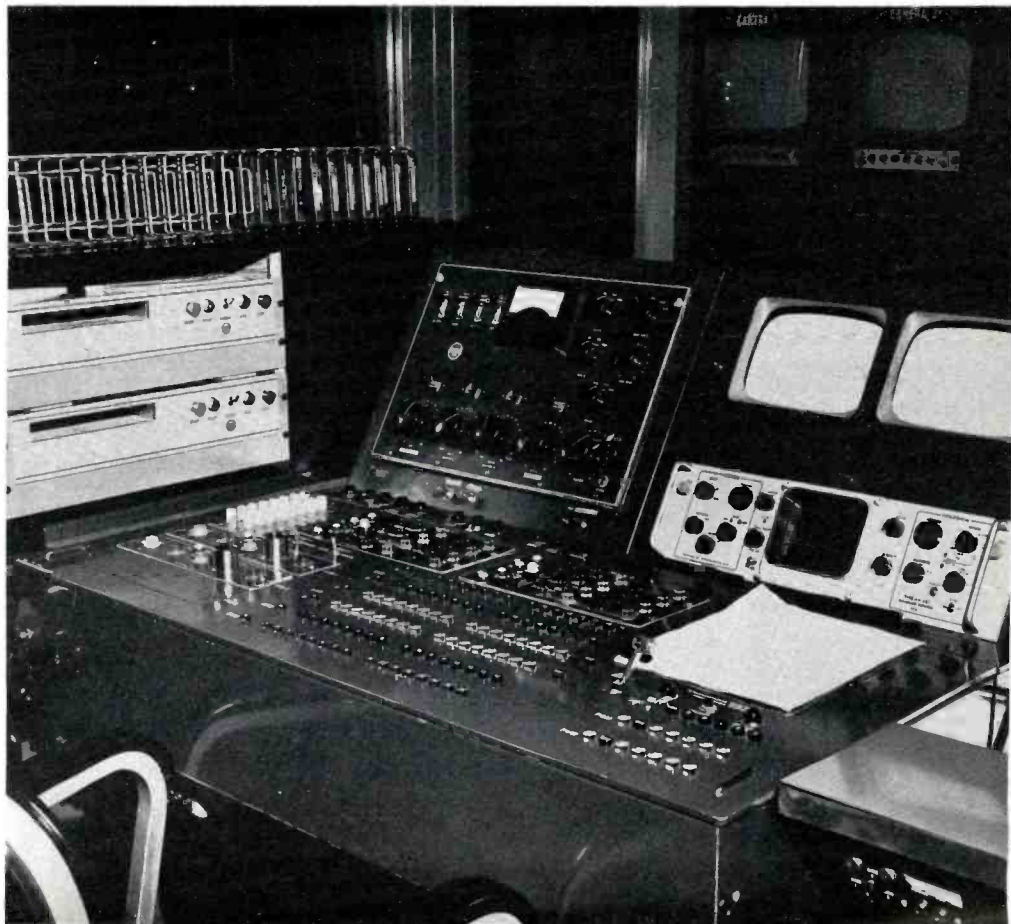
FIG. 8. (above) KCET Master Control includes a master switching position at the far left and film and tape control, right foreground. Monitors in back wall show individual camera outputs as well as studio outputs, tape outputs, line, etc.
