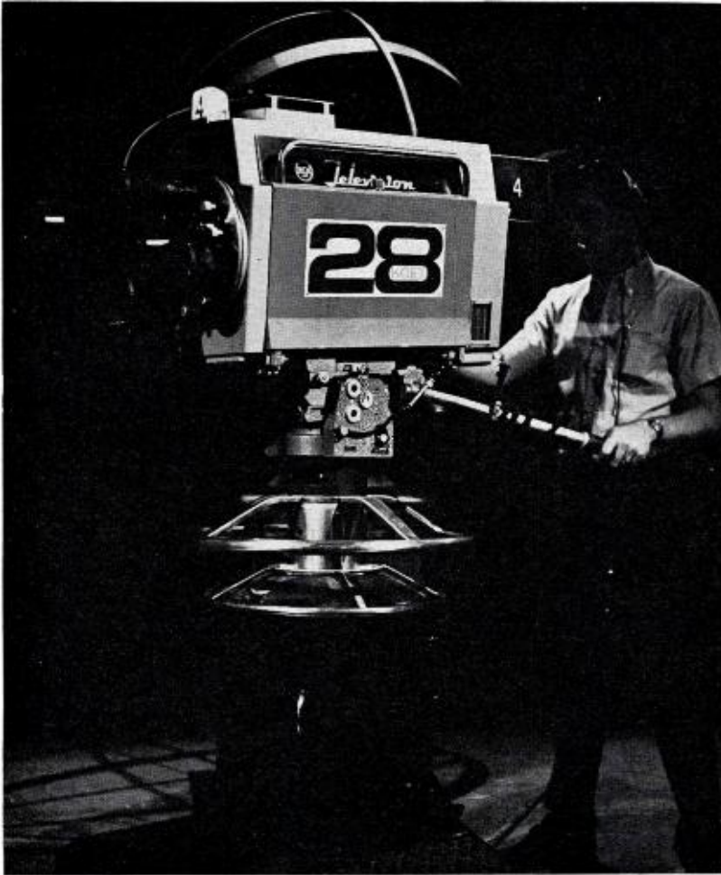
FIG. 1. In its studios KCET uses RCA TK-60 Deluxe 4½-inch Image Orthicon Cameras.
