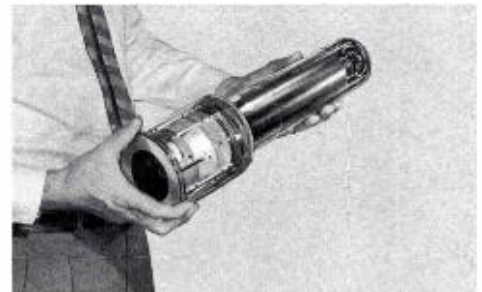
This is the big 4-1/2 inch I.O. tube for sharper pictures.
