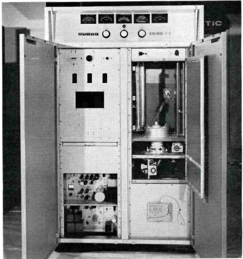
FIG. 2. All three transmitters—5, 10 and 20 KW—use same attractive cabinet, employ only two simple r-f stages following exciter. Optional FM stereo generator shown below exciter (at lower left).
