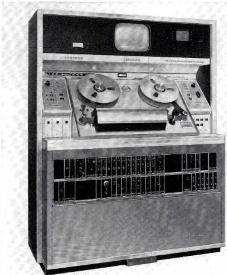
Modular layout of the deluxe TR-22. Many of these same modules are used in the TR-5, TR-4 and TR-3.
