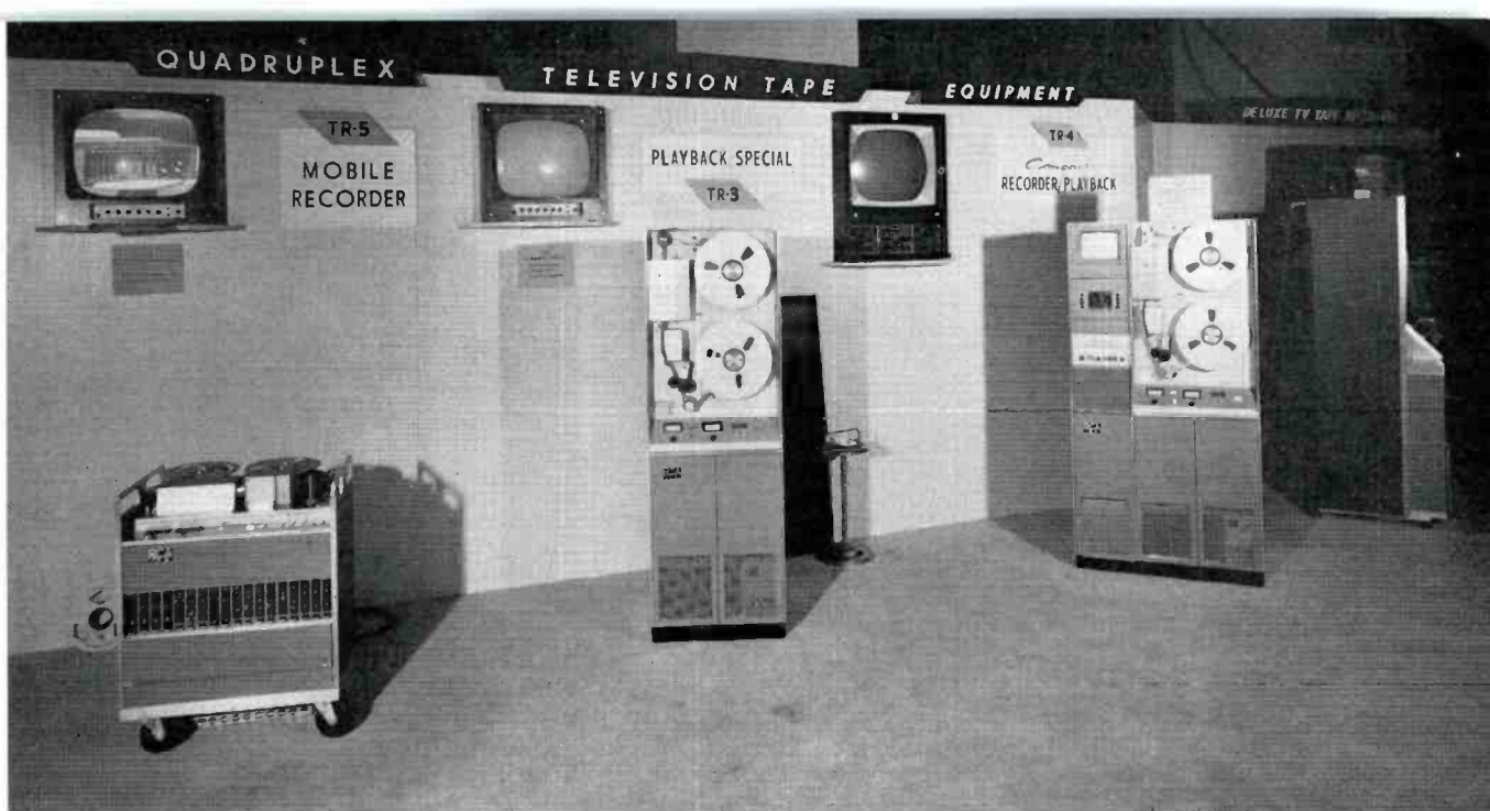
Three compact tv tape equipments . . . a TR-5 mobile recorder . . . a TR-3 playback machine . . . and a TR-4 economy recorder.
