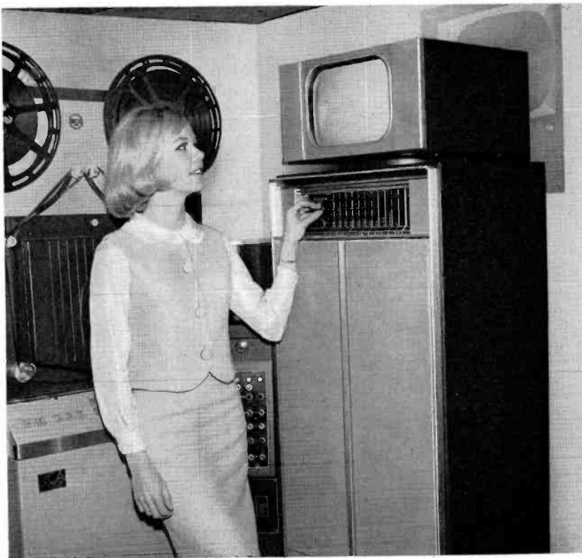
Complete 4-Vidicon Color Film Camera is contained in the stylish cabinet at right.
