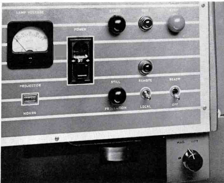
FIG. 6. A rotary switch is mounted below the projector control panel as shown here. By means of the switch the output from either the magnetic or optical preamplifier may be selected to feed the program line.
