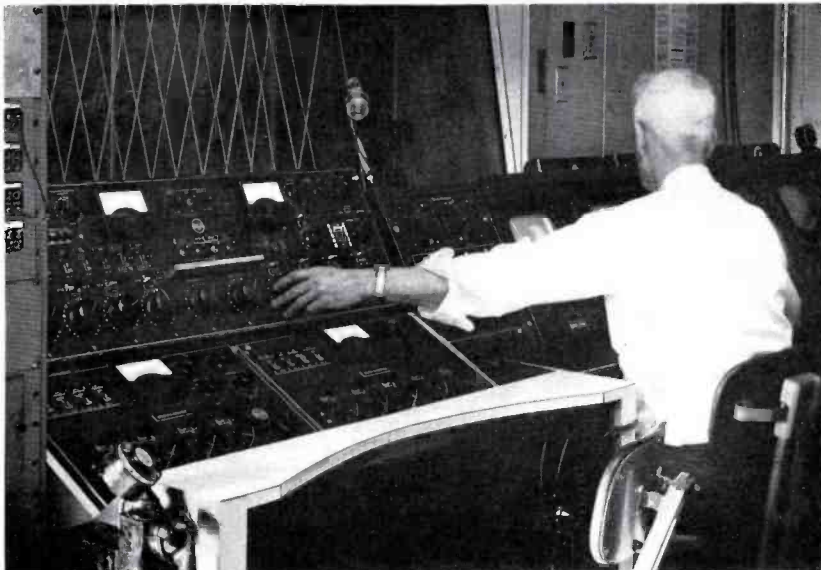
FIG. 5. One-man operation is illustrated here. During network and film periods the necessary audio and video controls are all within the reach of one operator.
