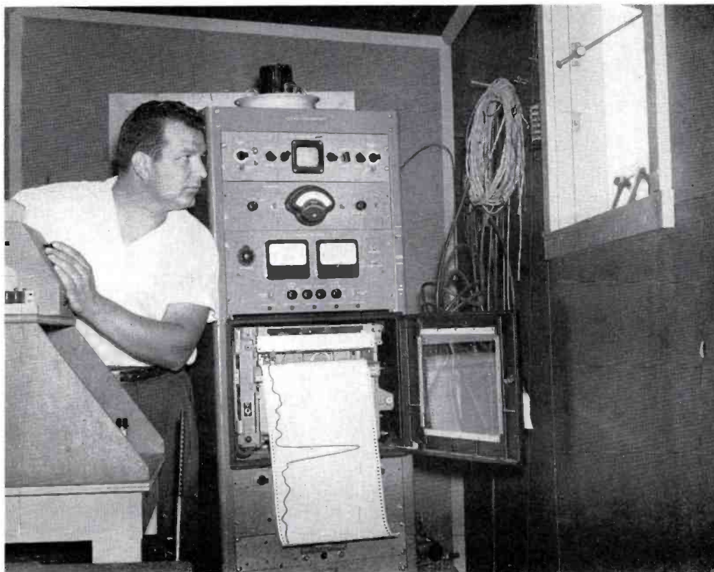
FIG. 9. As patterns of the antennas are measured they are continuously recorded as shown here. The speed and rotation of the turntables are also controlled from this location.
