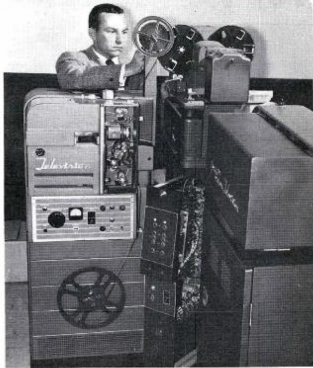
FIG. 4. Warren Happel, University of Michigan television engineer, inserts slides in TP-3 Projector. Also visible is the TK-26 Camera, TP-6 Projector and TP-15 Multiplexer.
