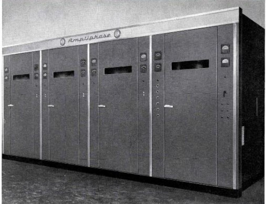
FIG. 1. This is the RCA Type BTA-50G "Ampliphase" Transmitter. Remote control system described in the article is ideal for this transmitter.
