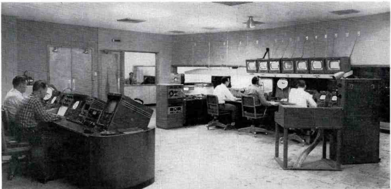
FIG. 11. Master control, at left, showing two operators. Studio control at right showing three operators, has following arrangement (left to right): tape recorder and microphone patch panel; two BQ-2B Turntables; audio control; director's position; video control, lighting.
