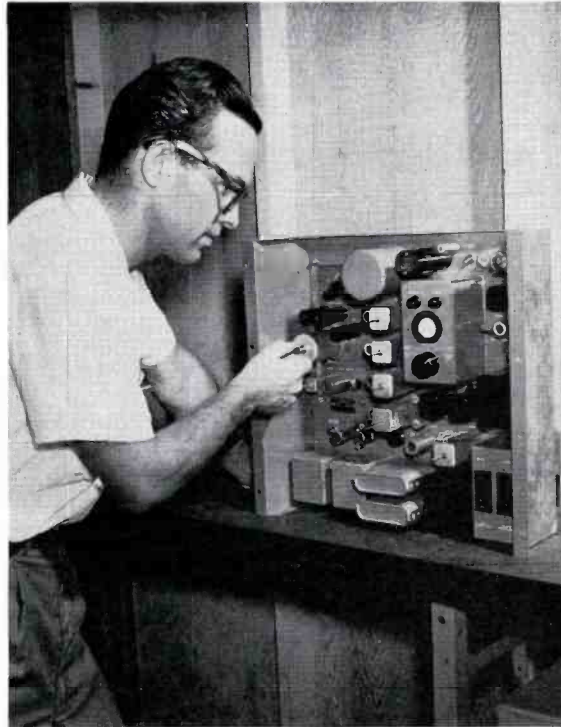
FIG. 10. All operating adjustments on the BTX-1A Subcarrier Generator are accessible from the front of the unit as shown here. Again the convenient built-in oscilloscope can be used to observe operation of AFC circuits. The author is shown checking divider circuits.
