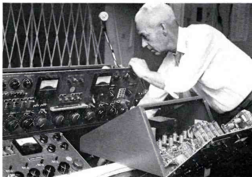
FIG. 7. The BC-5B Consolettes can be serviced by lifting up the front panel as shown here (or as shown in Fig. 8).
