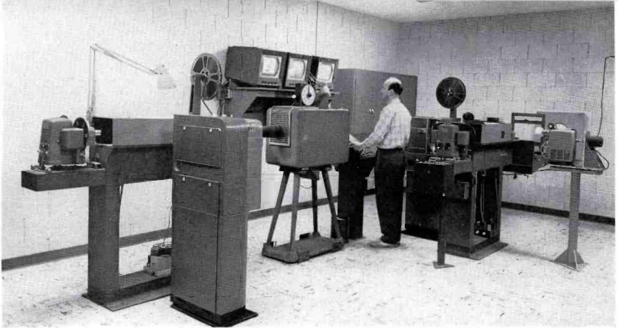
FIG. 16. KAKE-TV film room. There are two vidicon film chains, two TP-6 16-mm Projectors, two TP-11 Multiplexers, a telop, two TP-3C 35-mm Projectors. At far right, note 8-mm movie projector.
