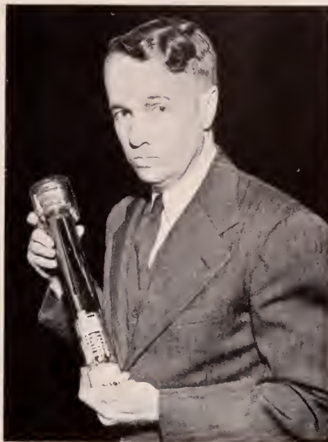
This is the "Aladdin's lamp of television"—the newly revealed super-sensitive camera "eye" known as the Image Orthicon.
